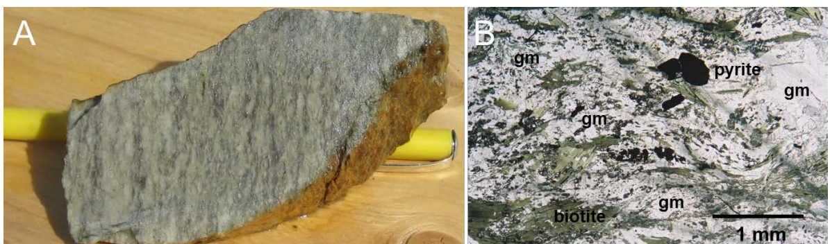
Figure 9: Felsic Schist in Drill Core and Thin Section
