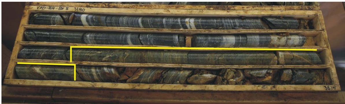
Figure 14: Core Box Photo of a Thin Ultramafic Sliver in CFD0164 from 31.8-36.14m
