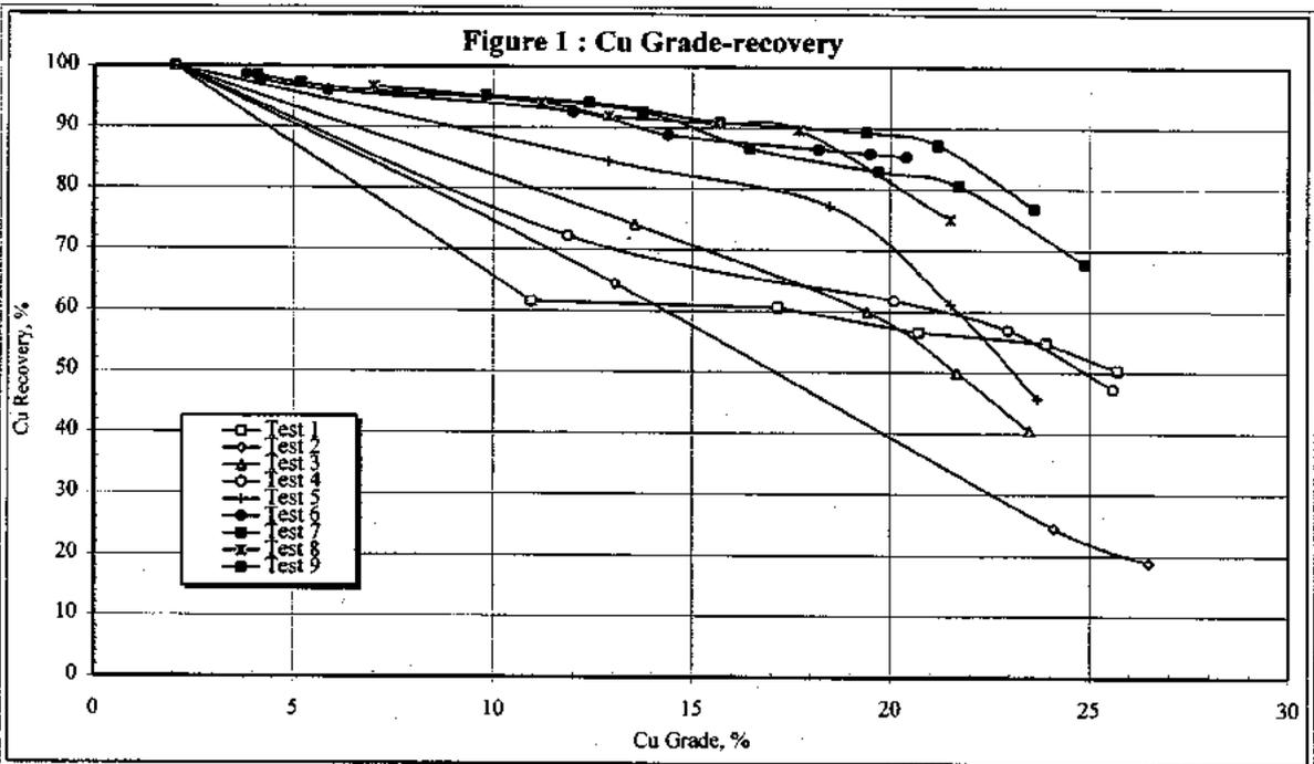
Copper concentrate of 20% Cu at 85-90% Cu recovery could be attained. Gold recovery was 60-65% at this grade.
