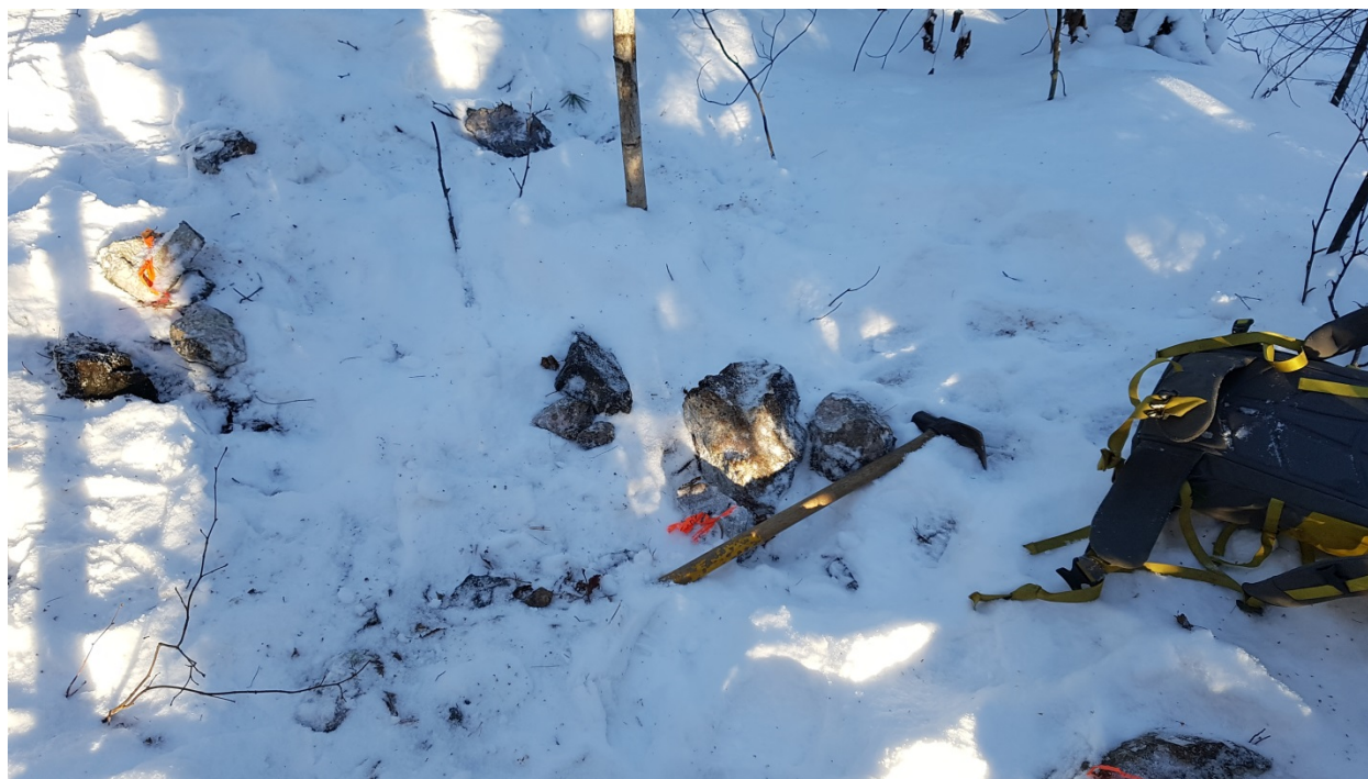
Figure 17 - Snow-covered muck pile near Shaft #1 at Shakt-Davis from which a verification sample was taken.
