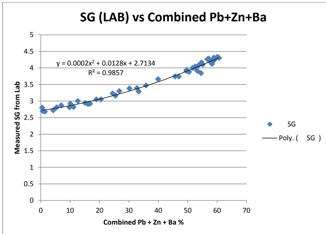
Figure 14.6: Scatter plot of Lab SG vs Combined Pb + Zn + Ba %
