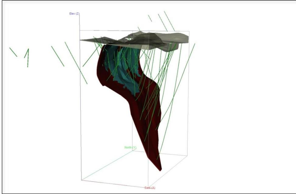
**Figure 14.2: Isometric view looking NW showing Mineralized Solid in red, Barite Shell in blue, surface topography, overburden surface and drill hole traces.**
