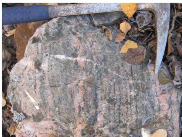
Fig. 9.12B Box mine area: K-feldspar altered biotite schist near contact with Box granite - partial "granitization".
