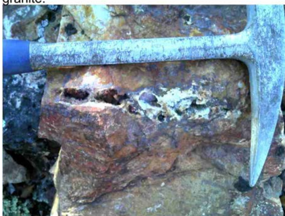
Fig. 9.13B Box mine area: Vuggy quartz veins filled with fine grained pyrite and trace chalcopyrite.
