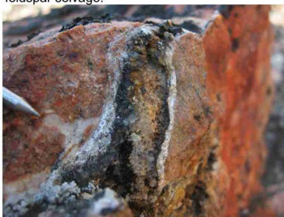
Fig. 9.12E Box mine area: rusty quartz+chlorite+pyrite filled vug/vein cutting Box granite. Note narrow white clay selvage..
