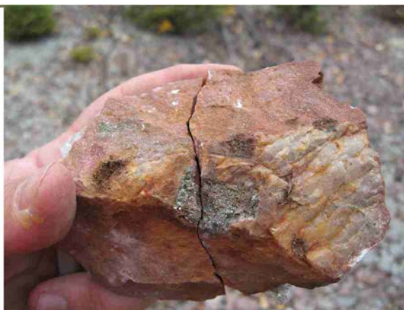
Fig. 9.13D Frontier adit dump: Cluster of fine grained pyrite on margin of quartz vein in f.g. pink granite?
