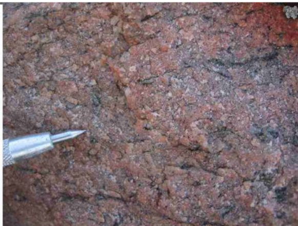
Fig. 9.11D Box mine area: fine grained altered granite. Difficult to distinguish from pink quartzite.
