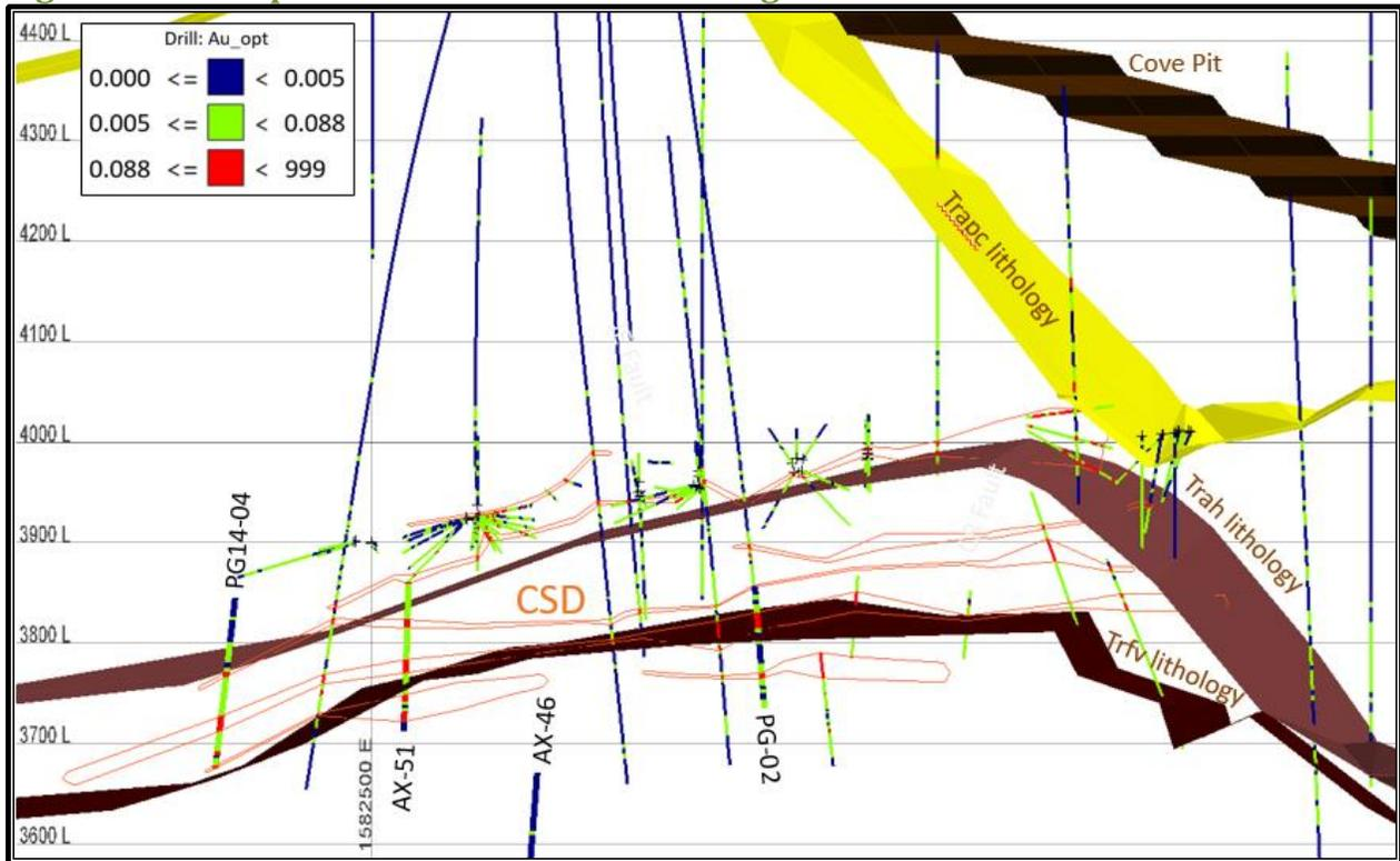
**Figure 10-5 Sample Section of 2201 Zone Drilling**
