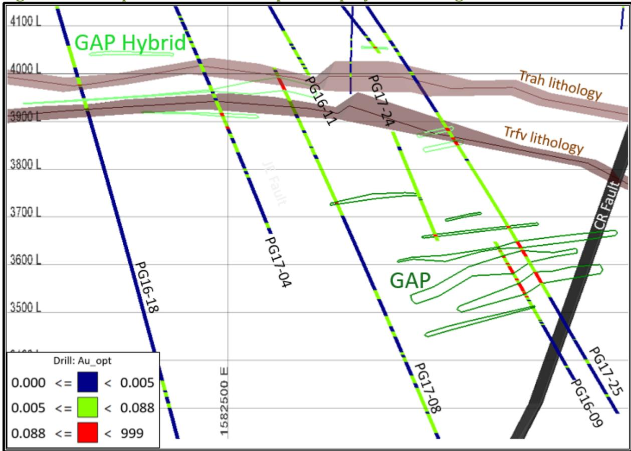
Figure 10-3 Sample Section of Helen Zone Drilling
