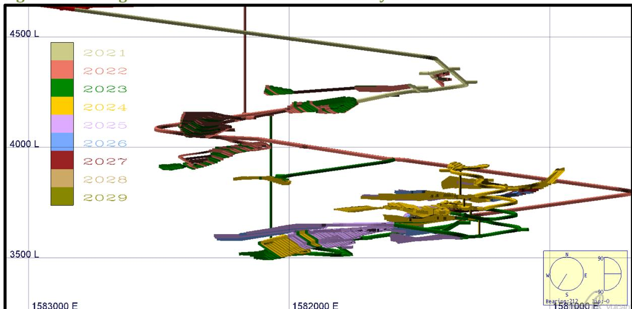
**Figure 16-8 Long Section View of Gap Mine Plan by Year**
