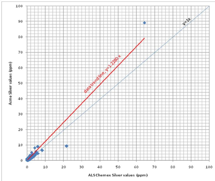
**Figure 14-8: Plot of ALS Chemex silver analyses versus Acme Labs silver analyses for field duplicate samples (2008, 2009 and 2010 data)**
