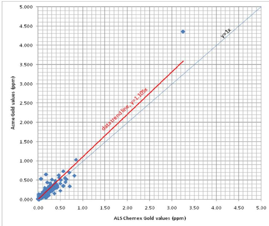
**Figure 14-7: Plot of ALS Chemex gold assay versus Acme Labs gold assay for field duplicate samples (2008, 2009 and 2010 data)**
