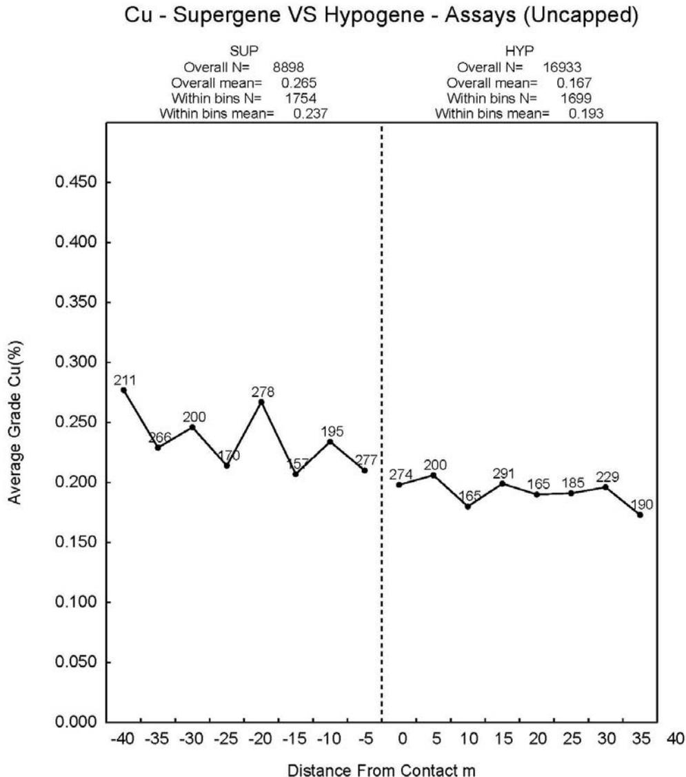
**Figure 17-3: Contact plot for Cu showing Supergene – Hypogene contact**
