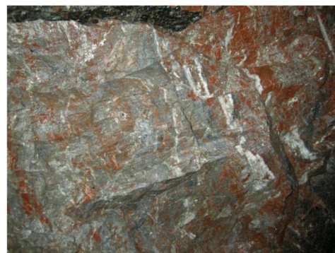
300 and 315 levels ore: massive pyrite-rich ?sericite-carbonate-?feldspar alteration, with reddish hematized wispy feldspathic domains and irregular quartz - ?albite-carbonate veinlets. Note lack of foliation in mineralization
