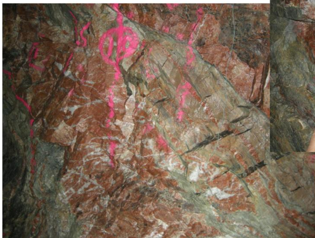
280 level south central: shallow dipping quartz extension veins preferentially exploit syenite-monzonite sills in Rusk Shear Zone. The veins are associated with auriferous pyrite aggregates within, and in clots peripheral to the veins
