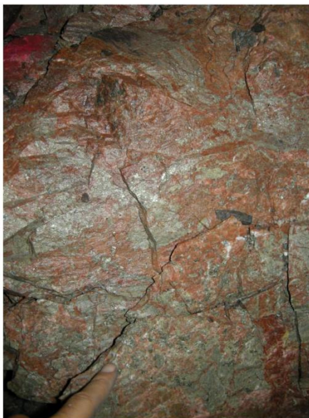
730 level: Rusk style massive pyritic sericite-bearing mineralization adjacent to monzonite contact in HW of Rusk Shear zone. Beside crosscut at approximately 4370E
