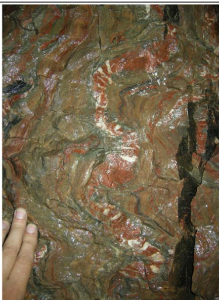
Late shallow dipping quartz veins occur preferentially in narrow syenite sills, cutting the shear zone fabric (left), but are also affected by the later set of folds with shallow dipping axial planes (D5) that overprint the shear zone (right), indicating that the folding is entirely post-mineral. 350 level crosscut (left, looking west)) and 280 level west crosscut (right photo, looking west)
