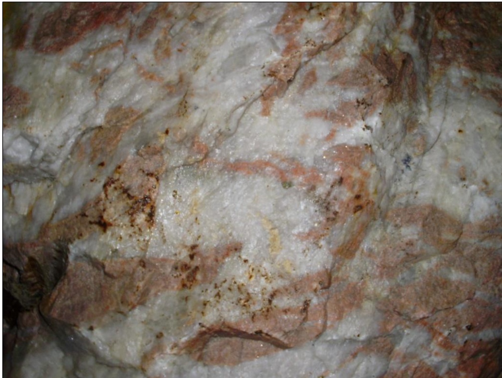
Plate 18: 715 Stope, Scheelite and Molybdenum in Quartz Veins Within Monzonite (D. Powers, 2011)
