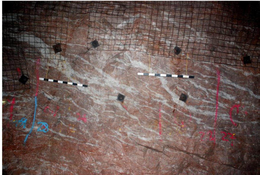
North wall, 730 level in Porphyry Zone within monzonite. Shallow easterly dipping sheeted quartz extension veins in central part of zone.
