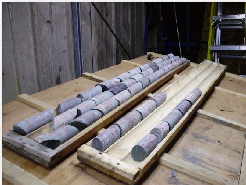
Plate 17 Condensed Diamond Drill Core, Archiving Drill Hole Lithologies
