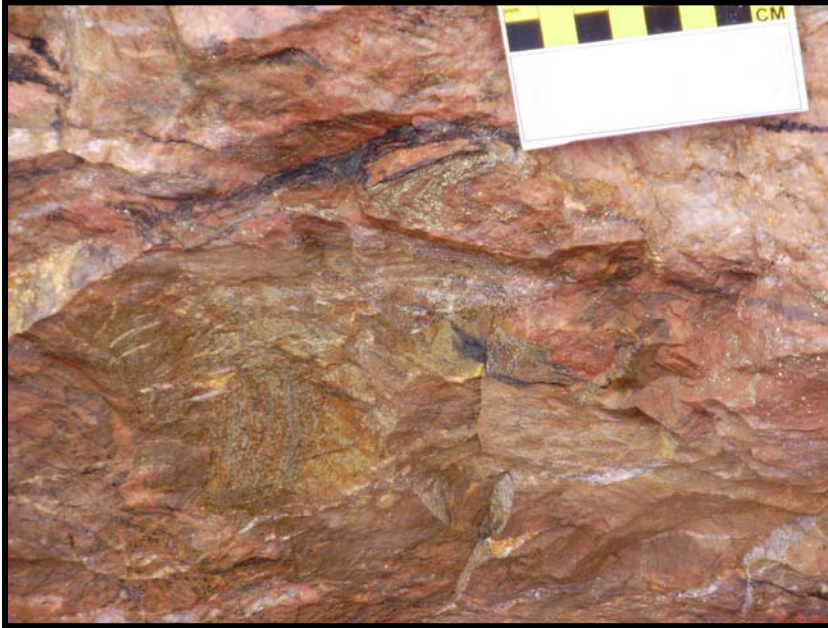
Plate 6., Area Five, Altered Alkali Intrusive Complex, hematite, iron carbonate, quartz +/- carbonate injections, sulphide (pyrite, chalcopyrite).
