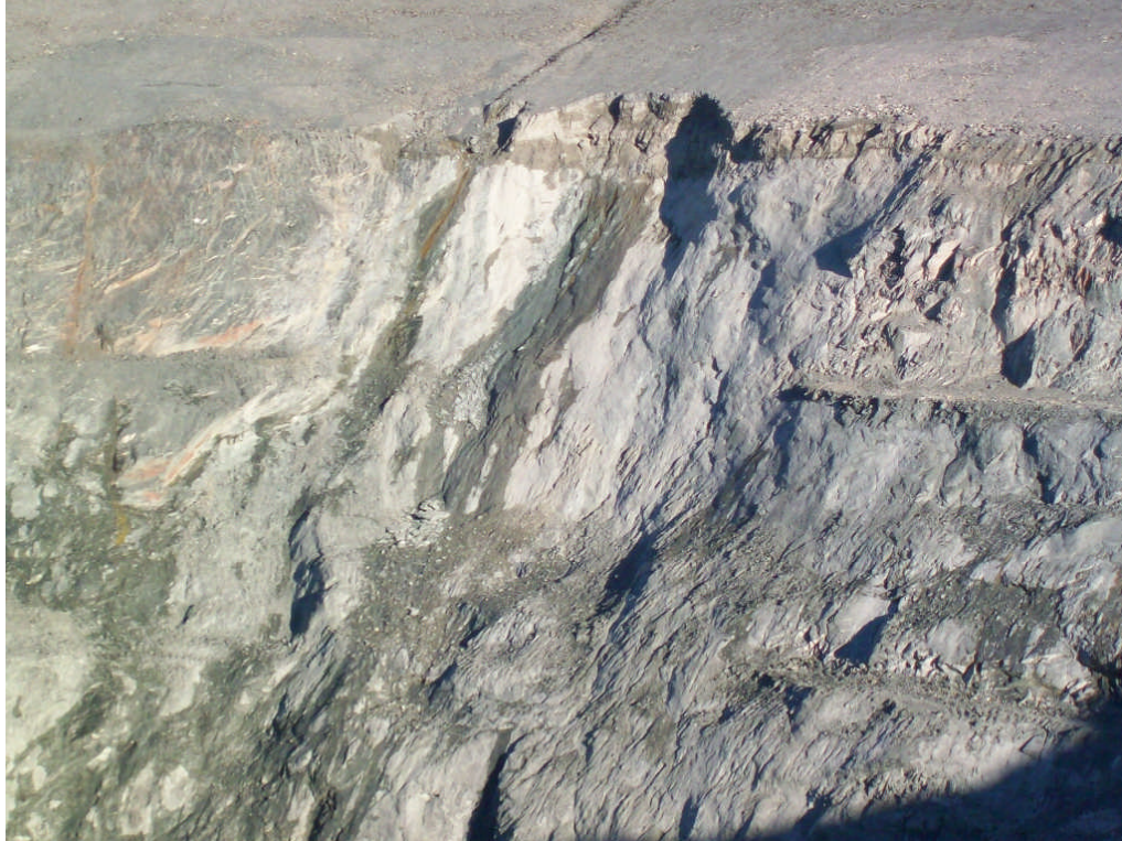
Figure 19.5 Seepage Along Overburden-bedrock Contact
