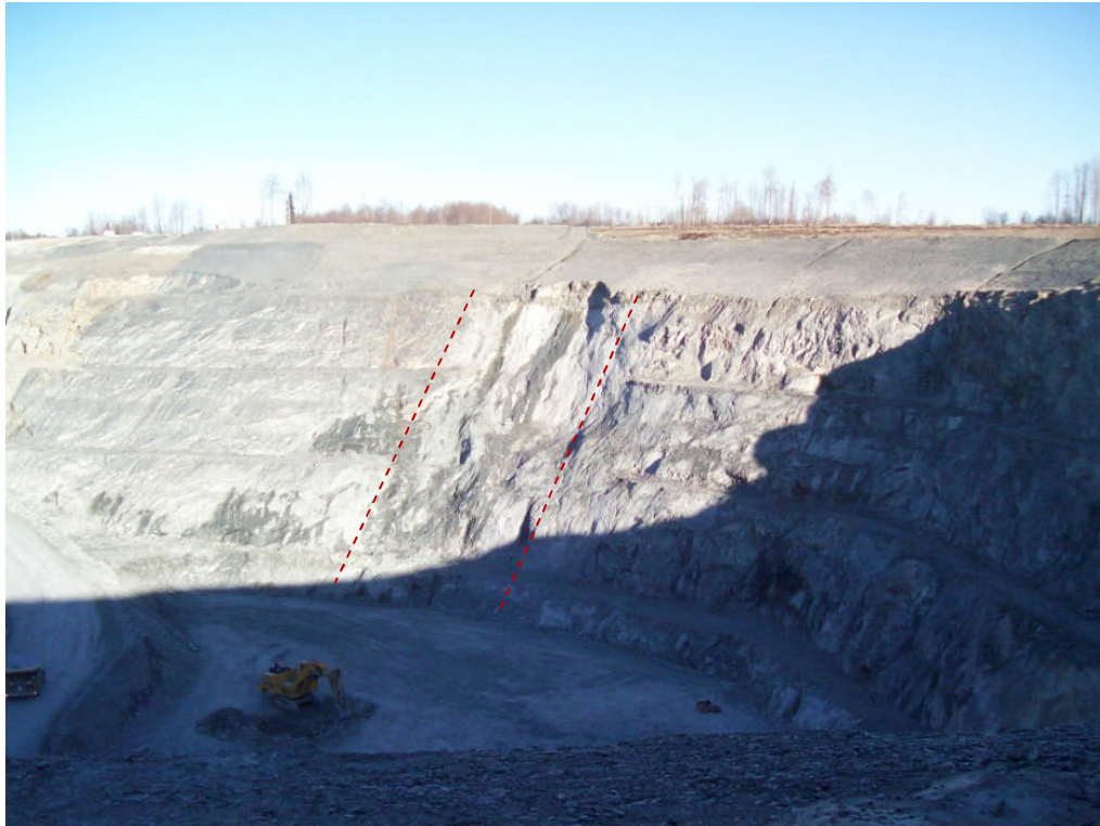
Figure 19.2 North Wall of Phase 1 Showing the Localized Shallow Planar Failure
