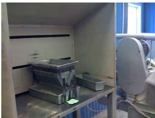
Figure 10-4: Sample riffle splitter (left) and pulverizer bowl (right).
