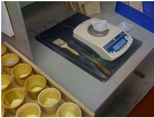
Figure 10-5: Assay lab samples assay balance (left) and cupellation (right).
