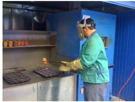
Figure 10-5: Assay lab samples assay balance (left) and cupellation (right).
