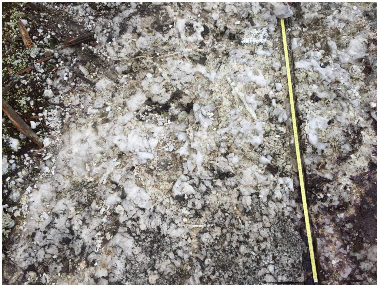
Figure 12-8 Photo of randomly oriented pale green spodumene crystals and grey quartz next to channel SC-03 on Main Dyke. Tape measure is within the channel cut and is 1.04 m long.
