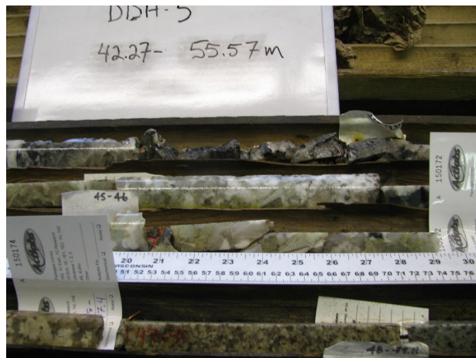
Figure 9-1 DDH-5 45-45.95 m with 3.24\% \text{Li}_2\text{O} (Power Metals, 2017 sampling)
