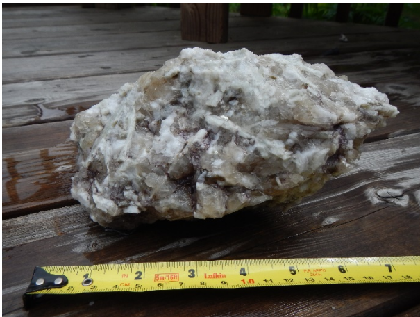
Figure 12-6 Main Dyke blast pit sample with pencil-shaped spodumene crystals.
