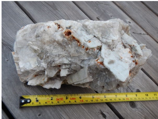
Figure 12-7 Main Dyke blast pit sample with knife-blade shaped spodumene crystals.
