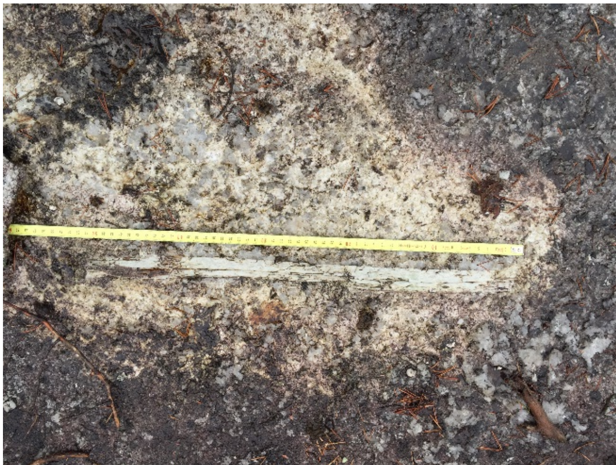
Figure 12-11 A 53 cm long spodumene crystal in a matrix of coarse-grained spodumene + grey quartz from North Dyke
