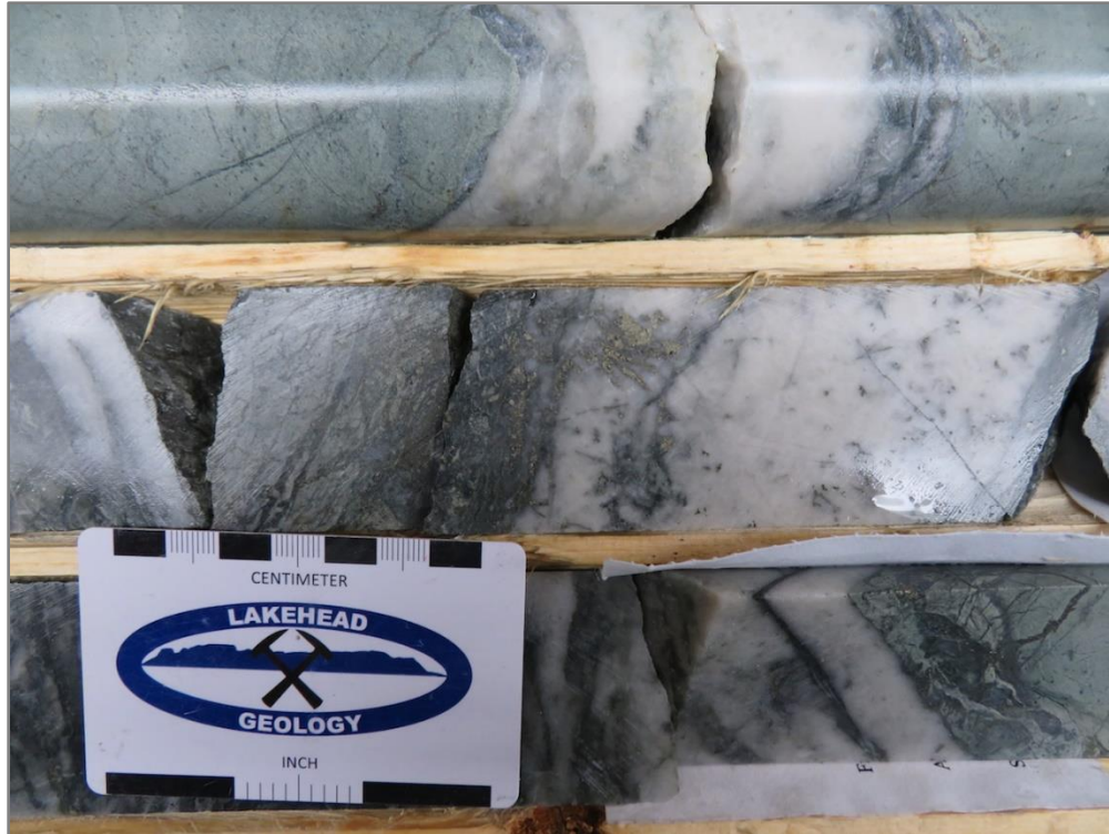
Photo 3 Hole RJK17-01 showing part of sample that ran 36.84 g/t Au / 0.5m at 120m
