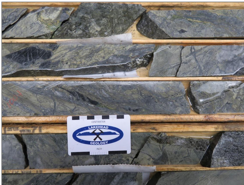
Photo 4 Hole RJK17-02 showing part of sample that ran 17.42 g/t Au / 0.9m at 100m
