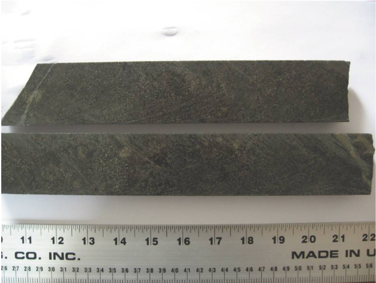
Figure 10: Semi-massive sulphide mineralization (primarily pyrrhotite and pentlandite) from drill core (H-07-48).
