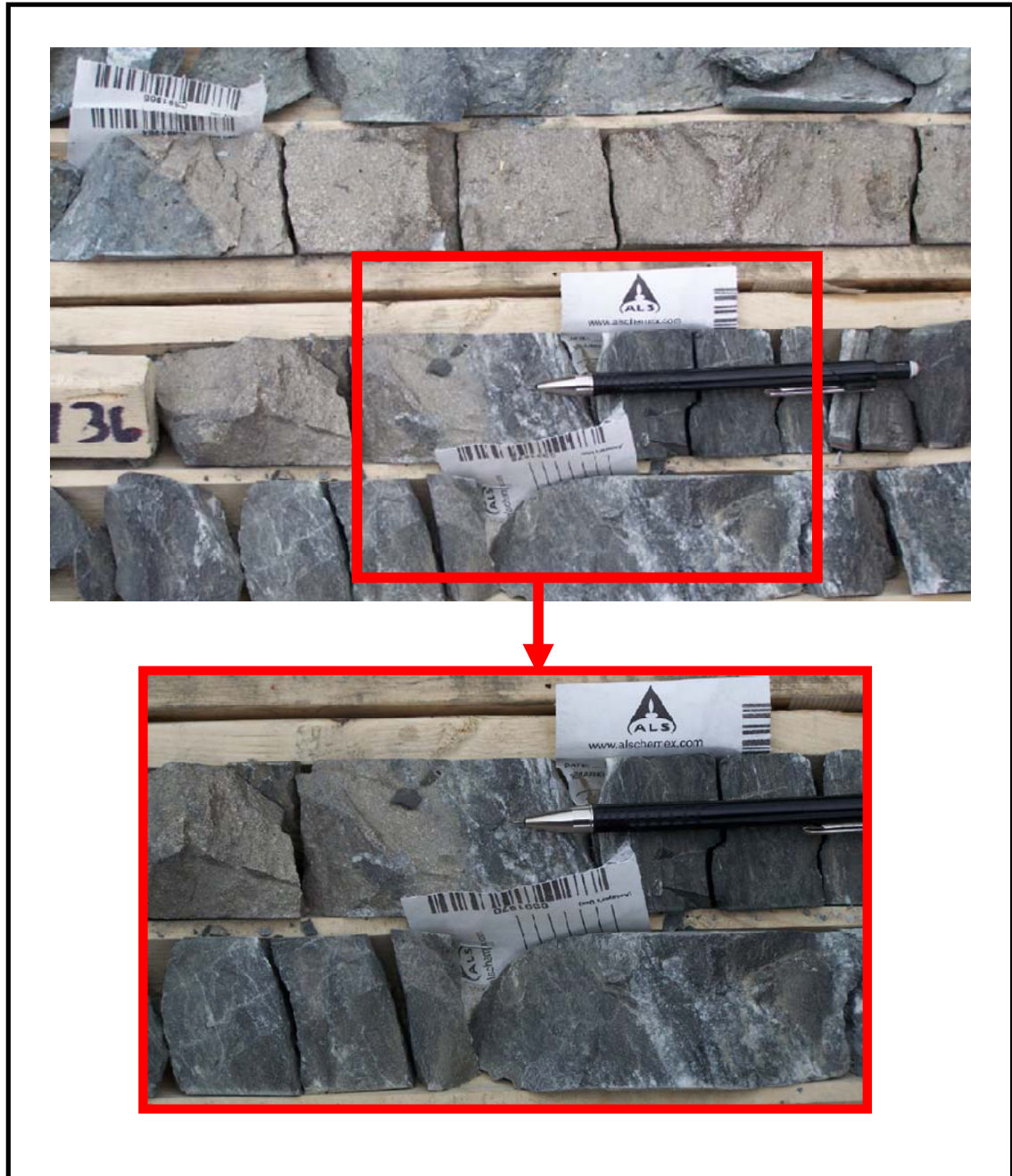
Figure 9: Structure associated quartz and carbonate veining at the base of the massive sulphide zone from drillhole RS07-6A.
