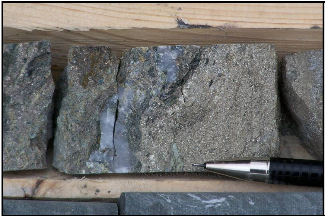
Figure 11: Massive sulphide mineralization (including pyrrhotite, pentlandite and pyrite) near the basal contact of a komatiitic flow and footwall dacite from drillhole RS07-6A.
