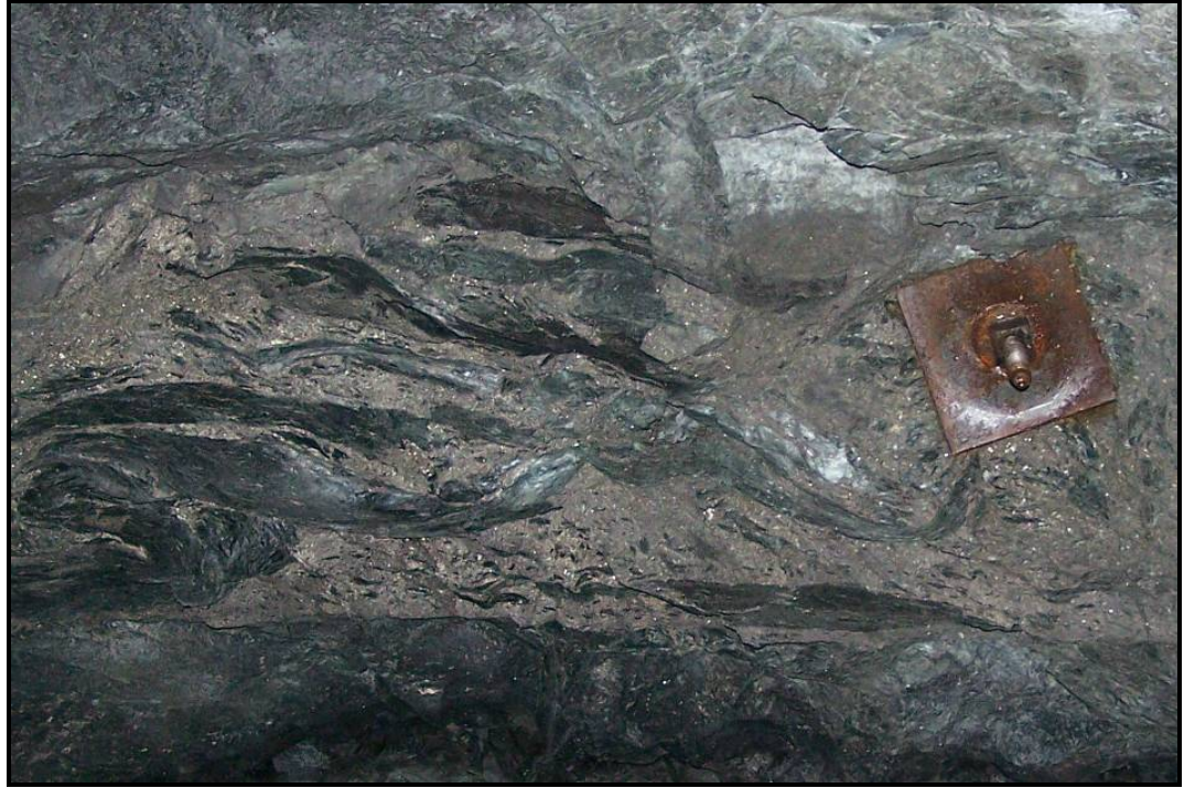
Figure 8: Durchbewegung texture within the massive sulphide deposit (fragments of wall rock preserved within ductile sulphide matrix)
