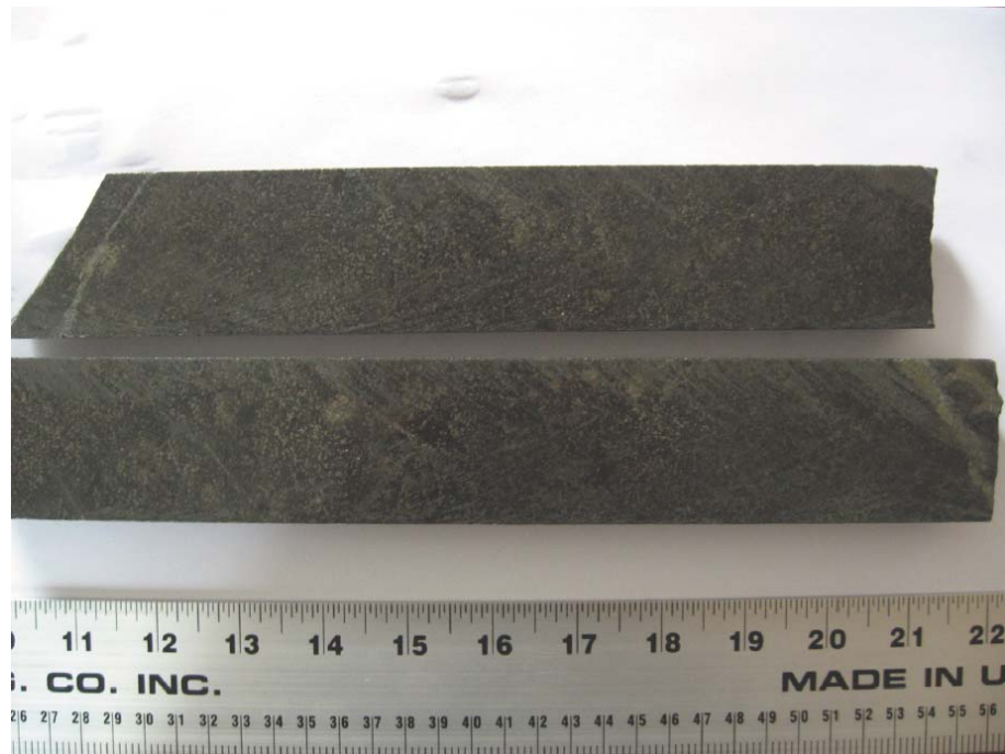
Figure 9. Semi-massive sulphide mineralization (primarily pyrrhotite and pentlandite) from drill core (H-07-48).
