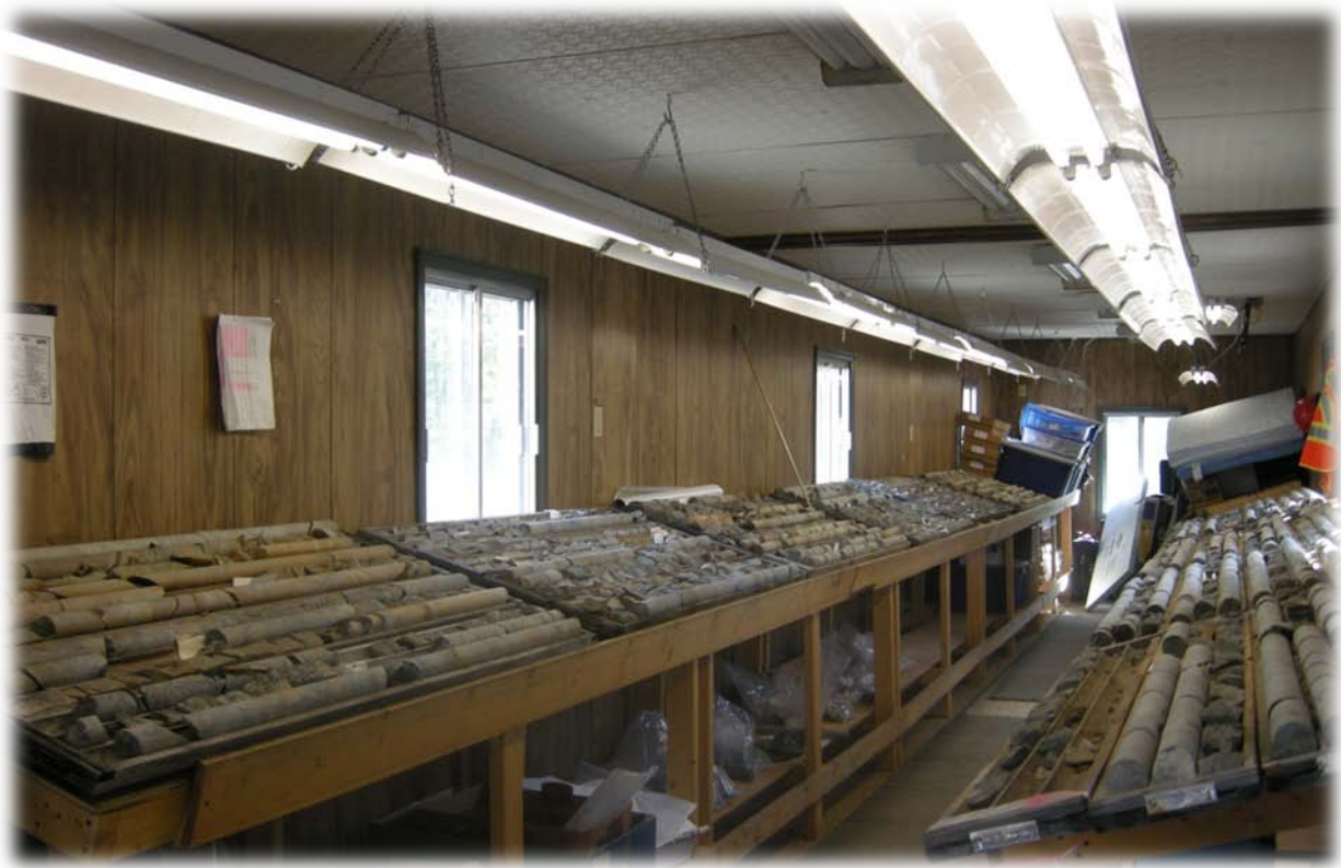
Plate 10-3: Creso core logging facility at Tyranite Mine.
