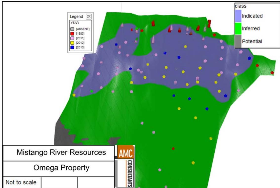
Figures 14.5 and 14.6 show the relationship between the modelled mineralized zones and the drilling data. The mineralized zones illustrated include blocks showing the estimated gold grades.
