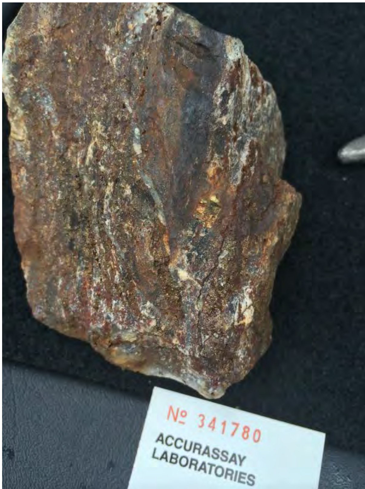
Figure 7: Emerald Lake Prospect: Sheared and silicified ironstone with pyrite after magnetite (replacement) and euhedral pyrite crystals in quartz veining. This sample assayed 3.32 g/t (check assay 2.9 g/t).
