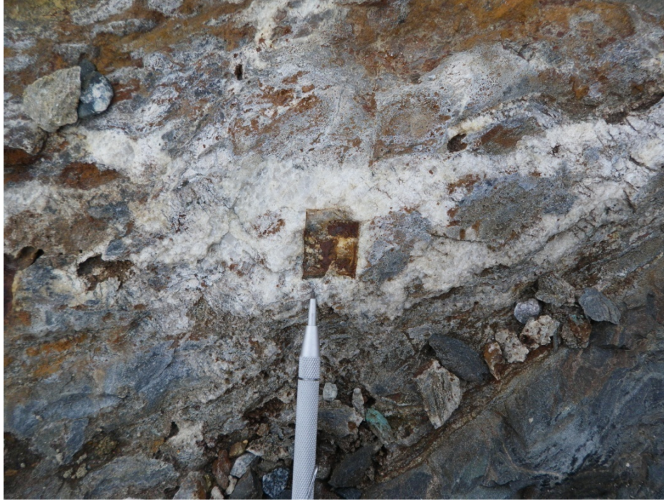
Figure 13: Oxidized mineralization in the main E-W shear Zone, with coarse to fine-grained pyrite boxwork.
