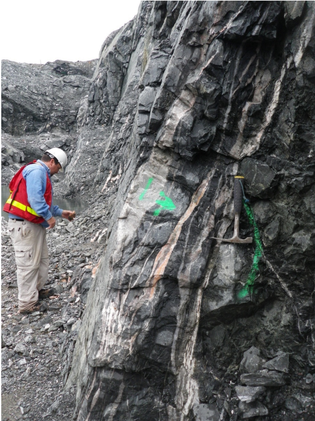
Figure 14: Main E-W subvertical structure with sheeted Quartz-Carbonate veins with fine-grained pyrite stringers.
