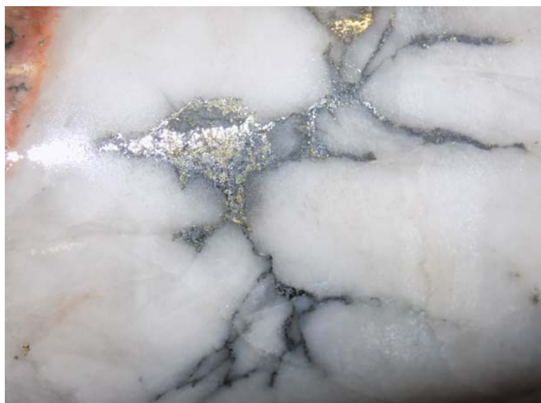
Figure 7-2 Au-Bi-Te stringers in quartz vein from 54.6 m, MG-14-12.
