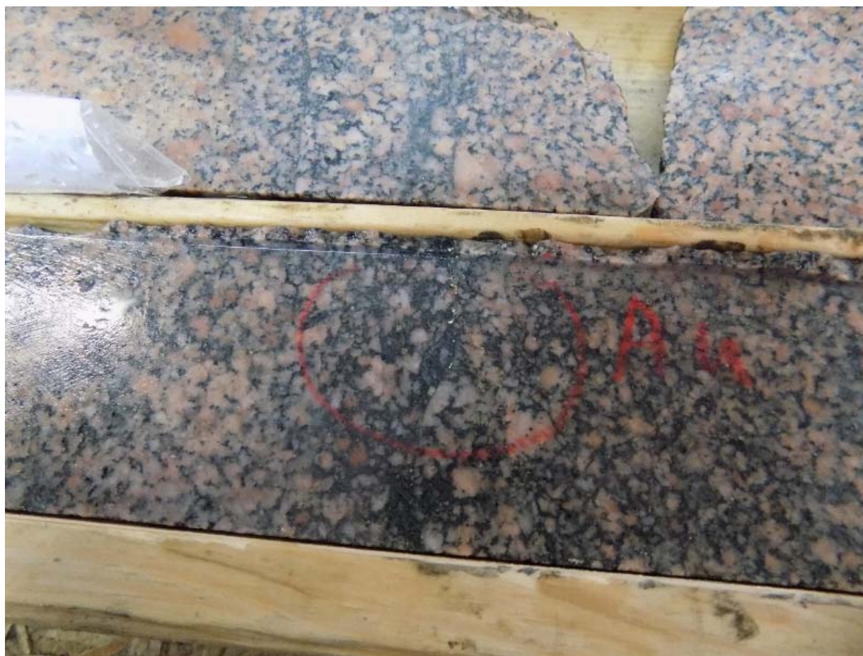
Figure 10-1 Drill hole MG14-09, NQ cut core containing visible coarse gold with black chlorite grains directly hosted in syenite, sample 14149 assayed 10.7g/t Au/1.0 metre.
