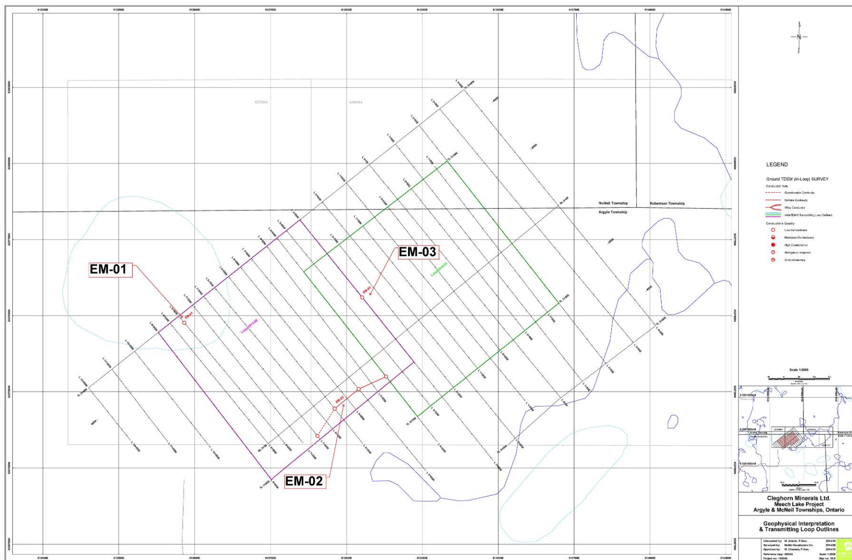
Figure 10: Meech Lake grid showing locations of TDEM anomalies and loop outlines.
