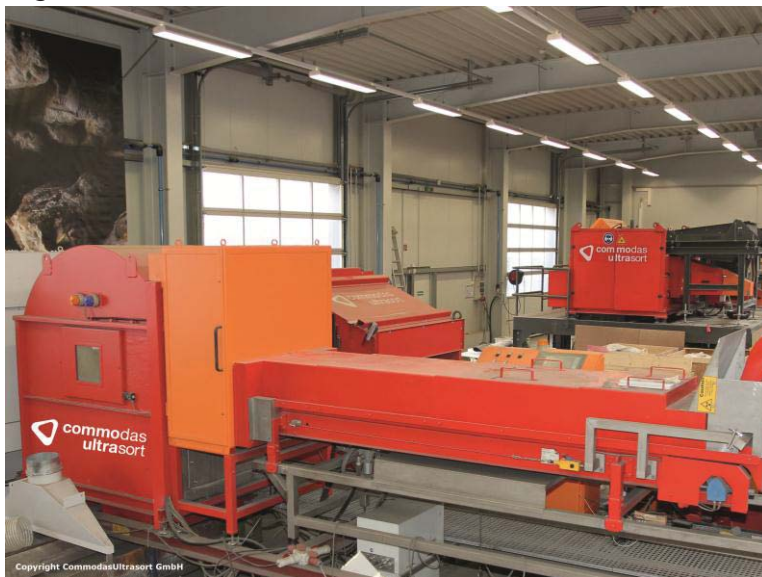
Figure 1: XRT Sorter used in the CommodasUltrasort test facility in Wedel, Germany.
