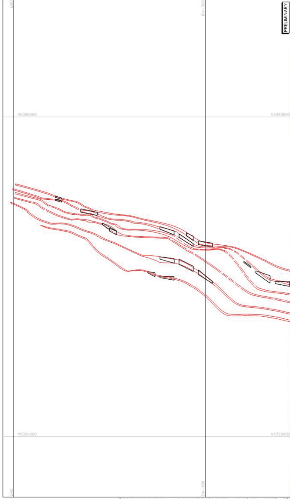
Figure 16.2: Mineralized Zone Section including Stopes (black): Section 486700 Looking East
