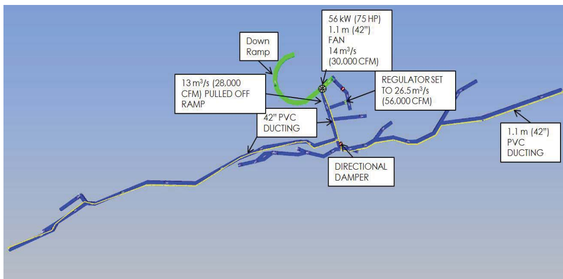
Figure 5.3: Typical Production Level Ventilation System
