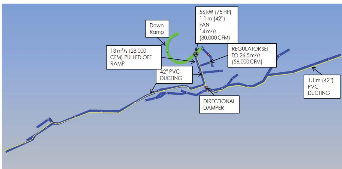
Figure 16.9: Typical Level Ventilation Circuit
