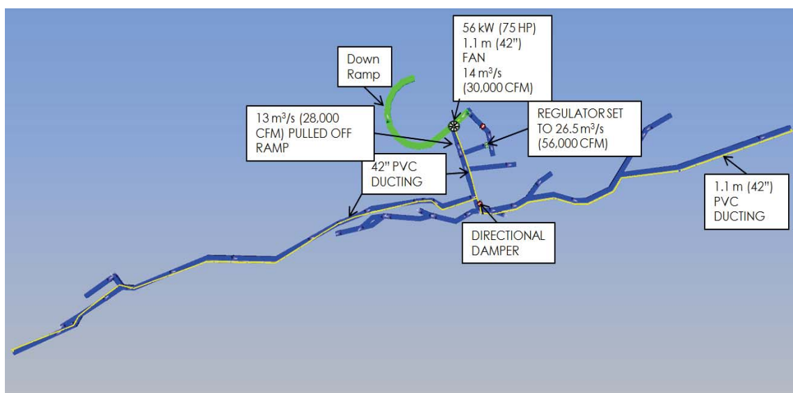
Figure 16.9: Typical Level Ventilation Circuit
