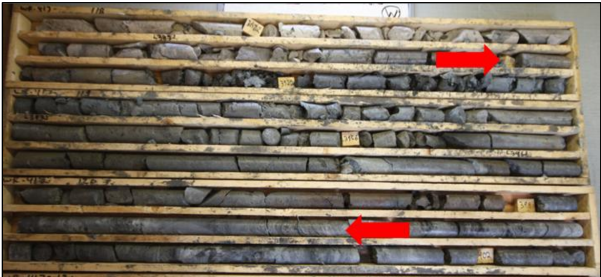
Figure 16-10: Poor to Fair Rock Mass Conditions in the Unconformity Domain (arrows indicate Phoenix mineralized zone)
