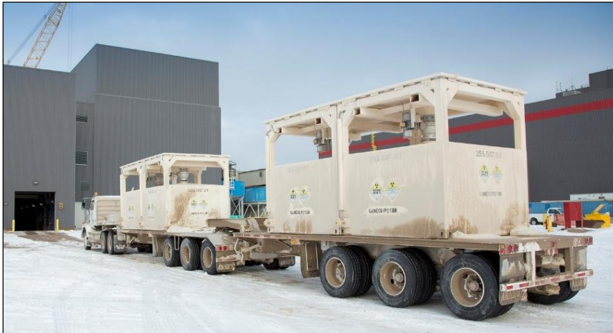
Figure 17-3: B-Train Tractor Trailer with Special Slurry Containers
