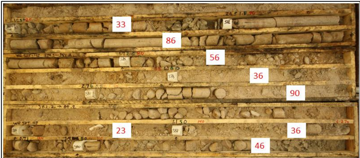
Figure 16-9: Poor to Very Poor Rock Mass Conditions in the Broken Zone Domain (% Core Recovery Shown)
