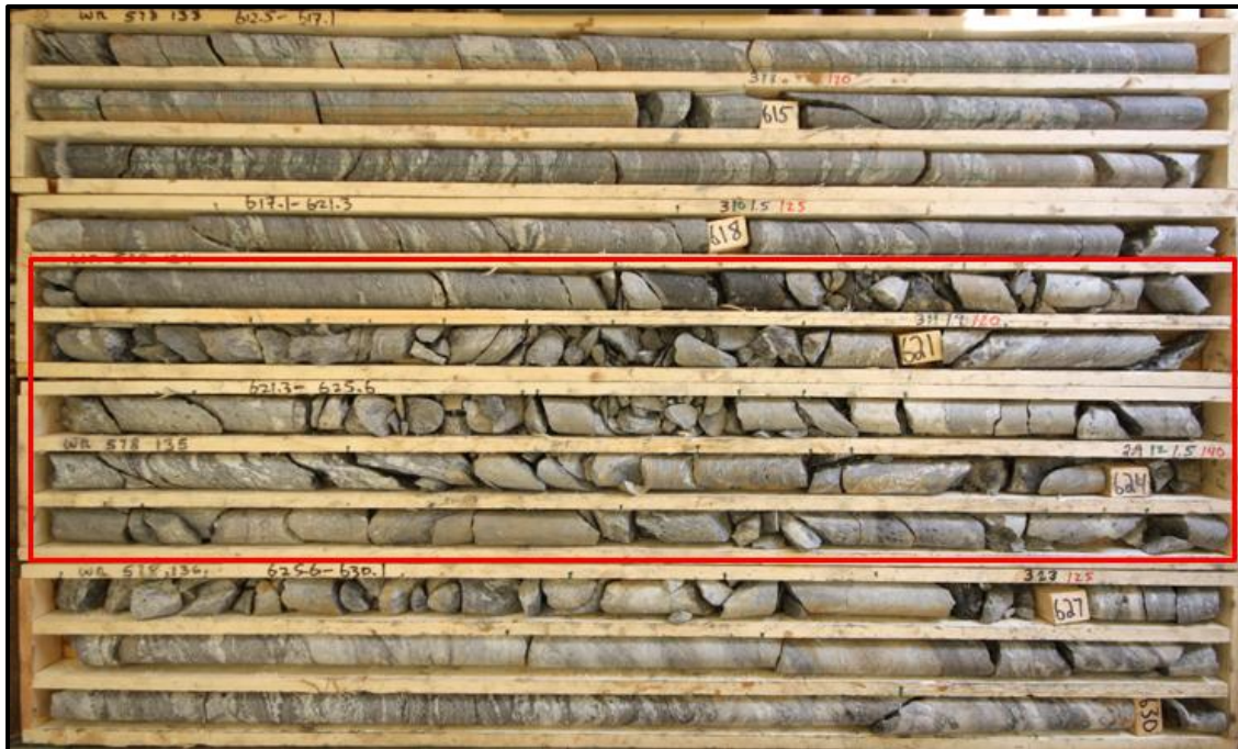
Figure 16-4: Example of Rock Mass Condition in the Gryphon Offset Fault (indicated by red box)
