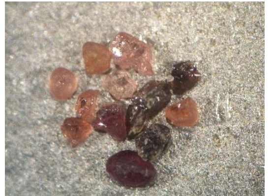
6 - The 2 purple grains microprobed are G11s – Garnets from till sample tested as magnetically inert
