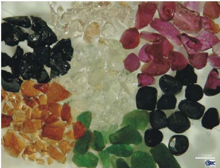
Photo F, “Kimberlite Indicator Minerals. From top left-clockwise: picroilmenite (Mg-rich ilmenite); eclogitic Fe-Mg-Ca almandine G3 garnets; peridotitic chrome pyrope G9/G10 garnets; chromites; chrome diopsides; Ti-Cr-Mg pyrope G1/G2 garnets; and olivines in the centre” (Quirt, 2004, p 2).
