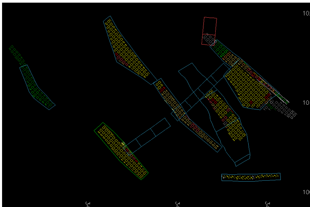
Figure 15-1: Example of Reserve Stope Design (Plan View)
