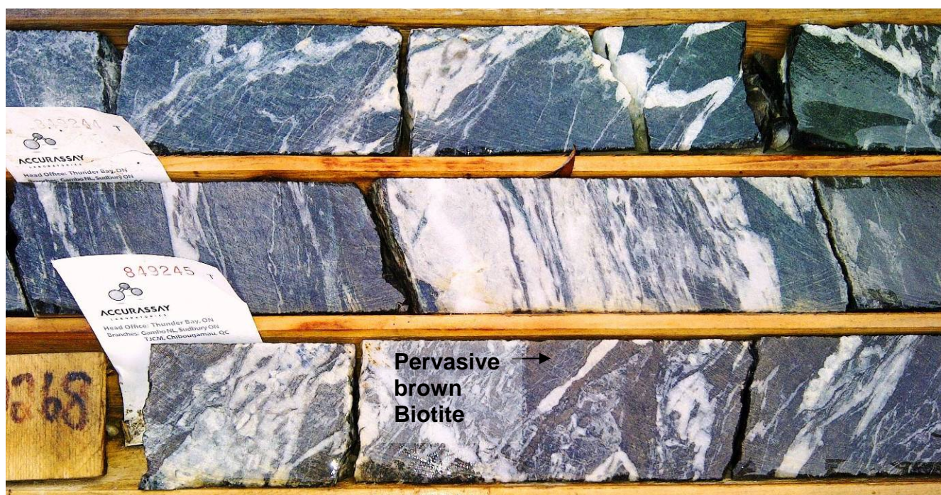
Figure 14-1: Strongly altered and sheared zone in Balmer basalt at 2268 m, MH1103.
