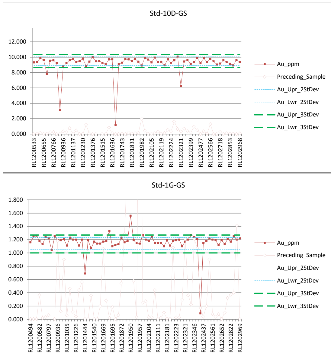
Time series plots for Blank and Certified Reference Material Samples Assayed by SGS Laboratory during 2012 drilling program.
