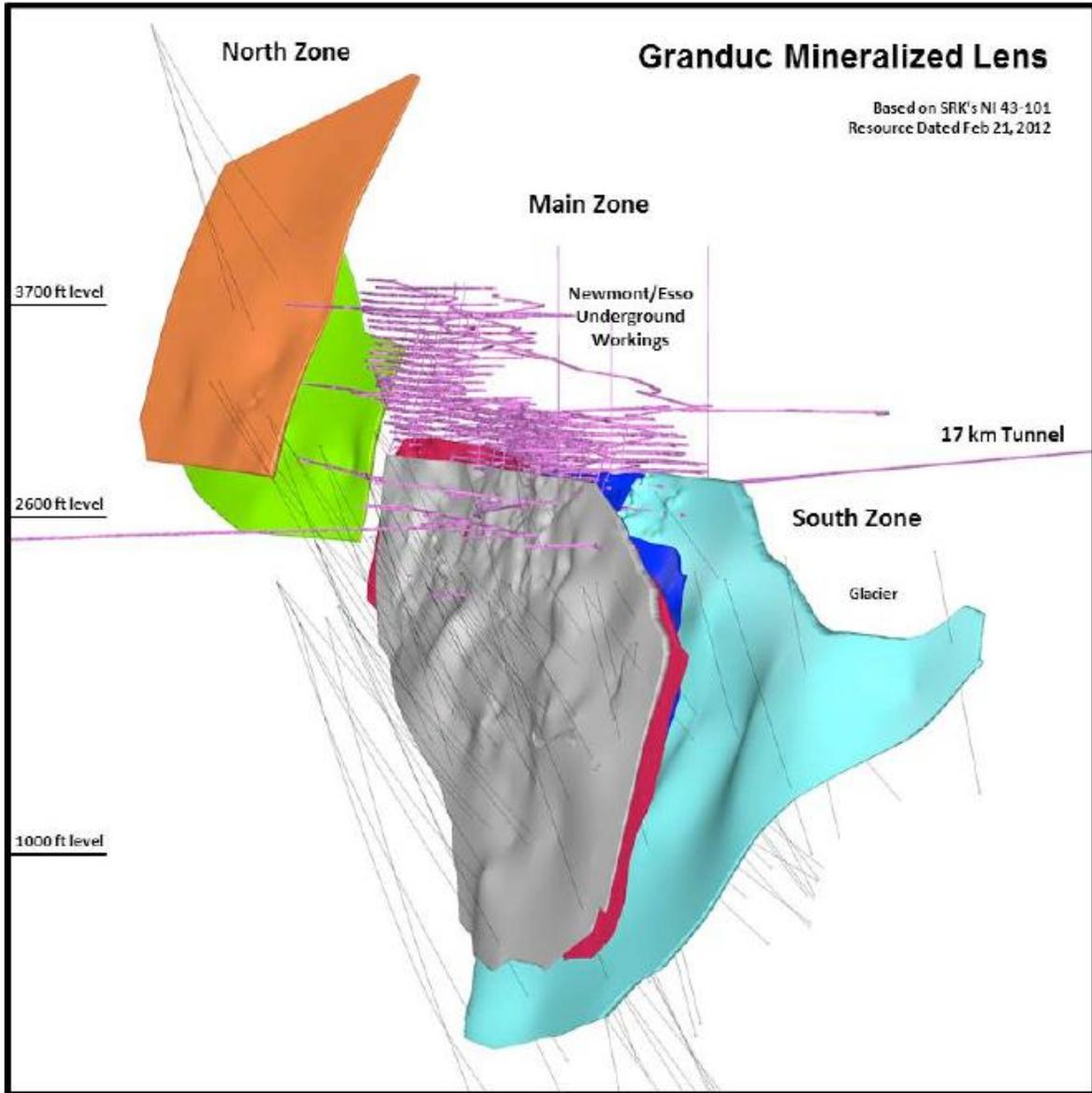
**Figure 13.2: Isometric View of Interpreted Main, South and North Domains**
