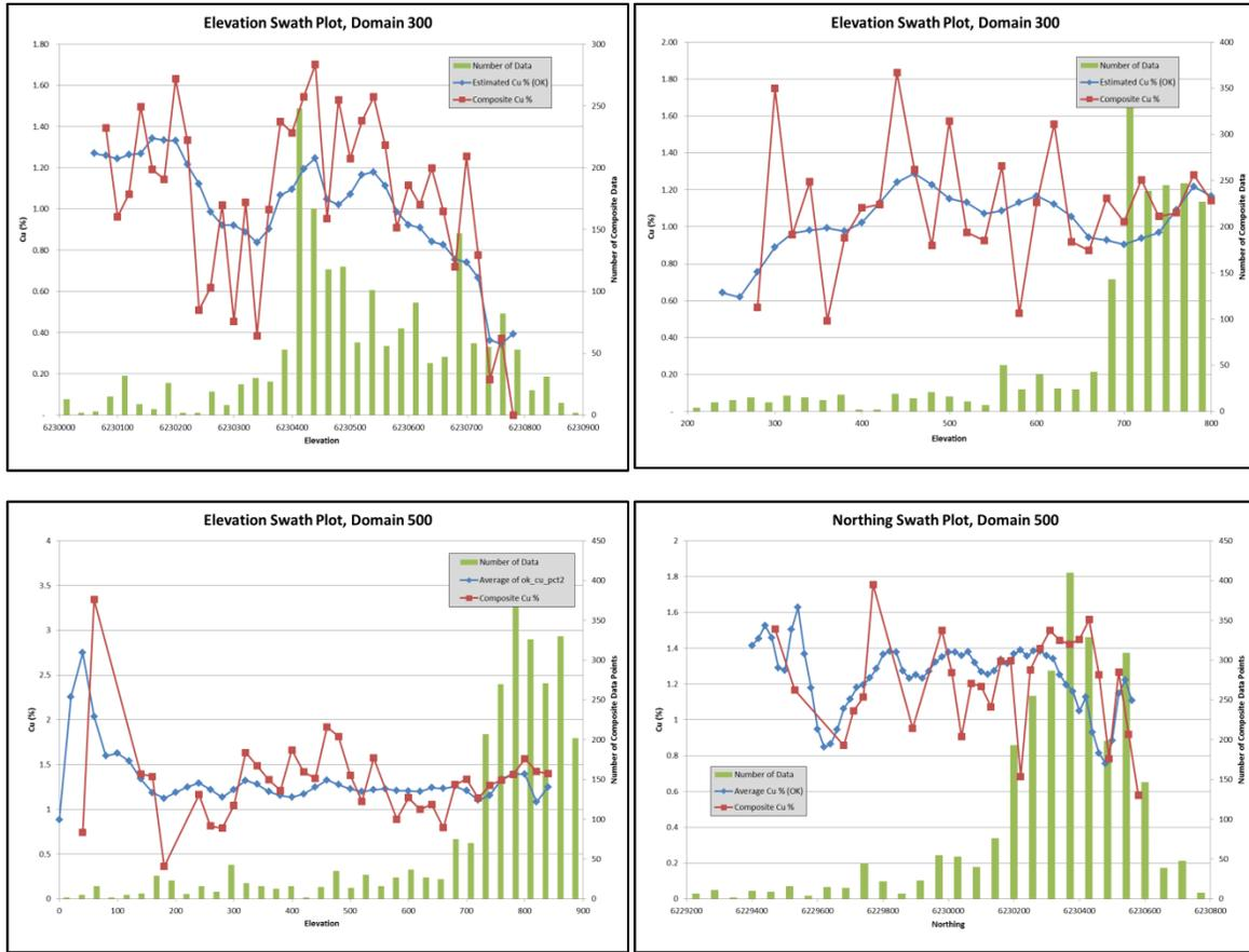
**Figure 13.10: Z (elevation) and Y (Northing) Swath Plots for Domain 300 (top) and 500 (bottom)**
