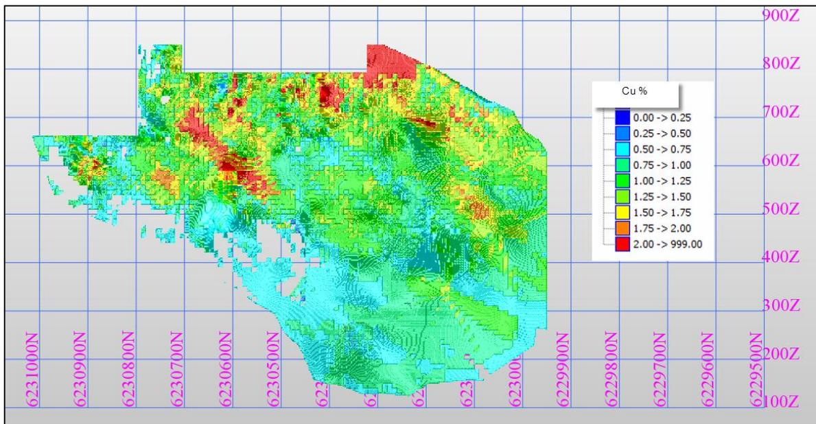
**Figure 13.6: Domain 100 in Long-Section Showing Cu Grade Variation.**
