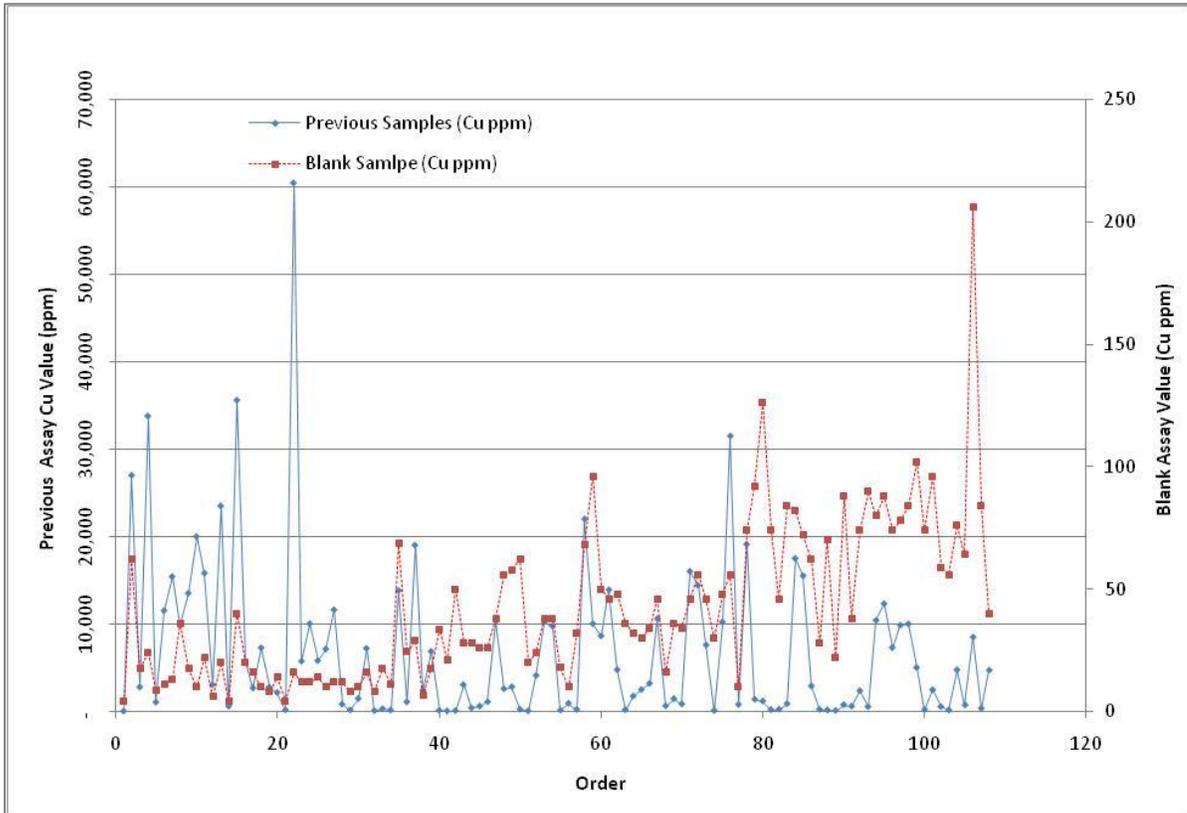
**Figure 11.6: 2010 Blank Sample Values Compared to Values of Previous Samples**
