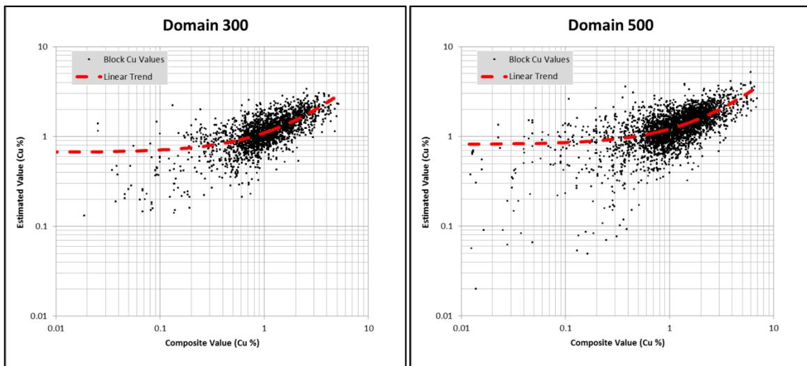
**Figure 13.9: Comparison of Block Estimates with Composite Data within the Blocks for Lenses 300 and 500**
