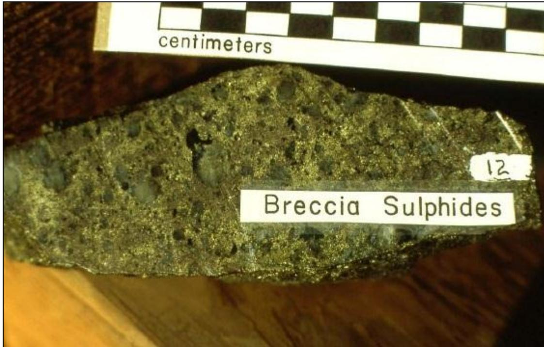
**Figure 7.3: Remobilized Pyrrhotite-Chalcopyrite with Brecciated Mafic Tuff and Chert
