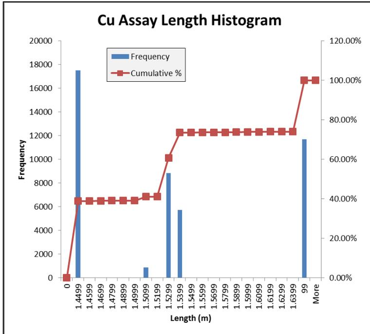
Figure 13.3: Histogram of Sample Lengths in the Mineralized Zones
