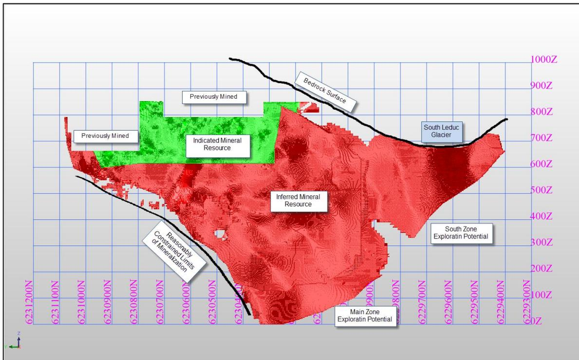
**Figure 13.8: Long-section of Main Zone Block Model Highlighting Mineral Resource Classification**
