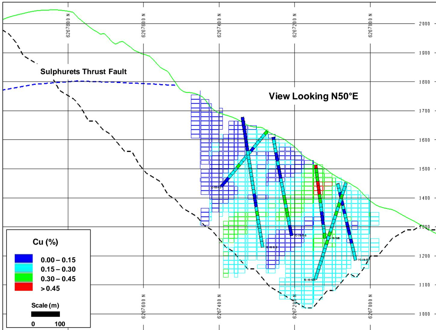
Figure 17-35: Iron Cap Au Block Model - 1395 Level
