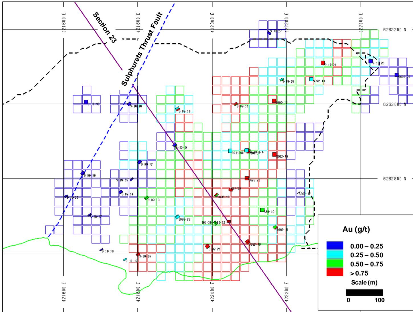
Figure 17-28: Sulphurets Cu Block Model - 1275 Level
