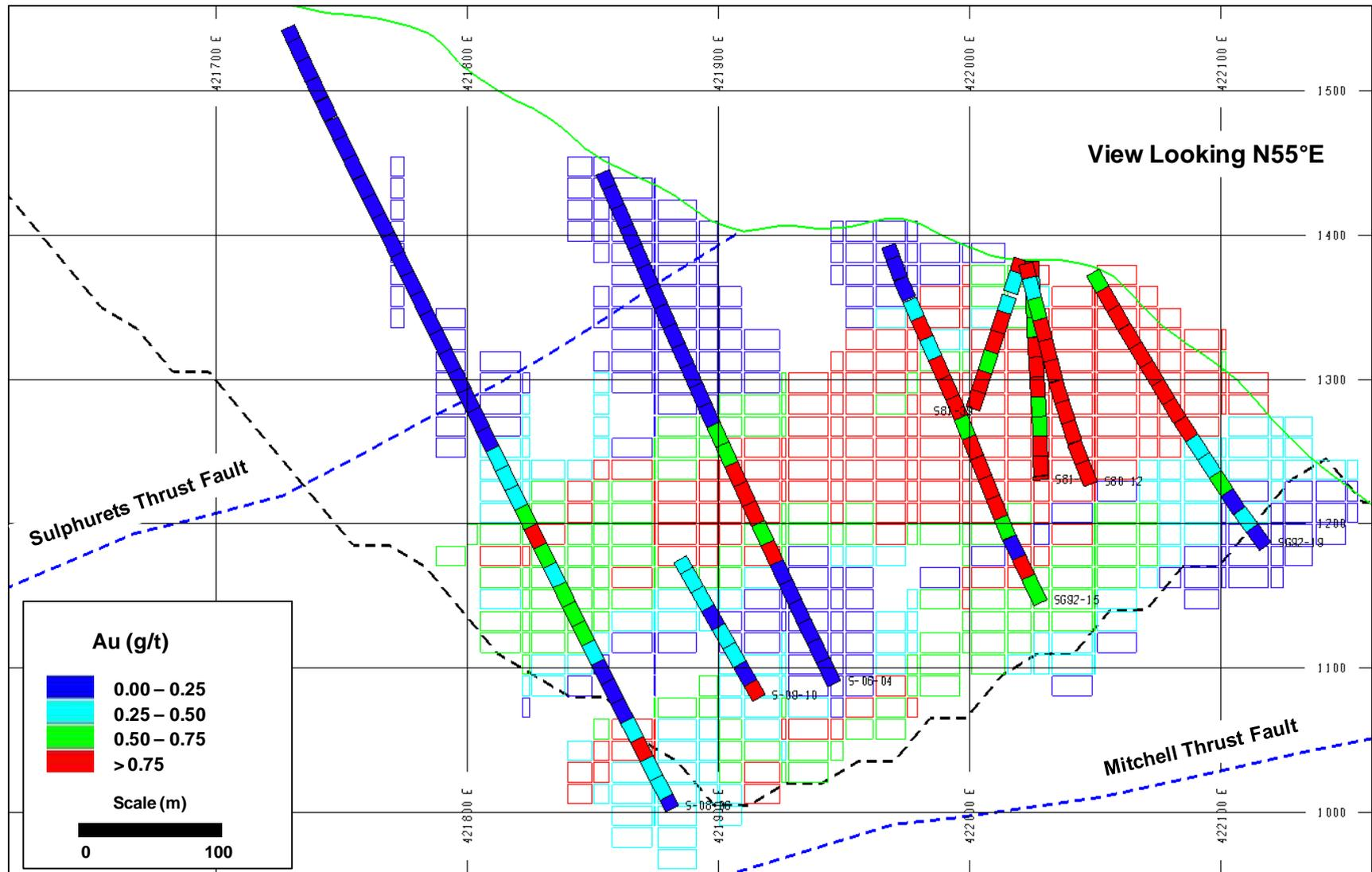
Figure 17-26: Sulphurets Cu Block Model Cross Section 23
