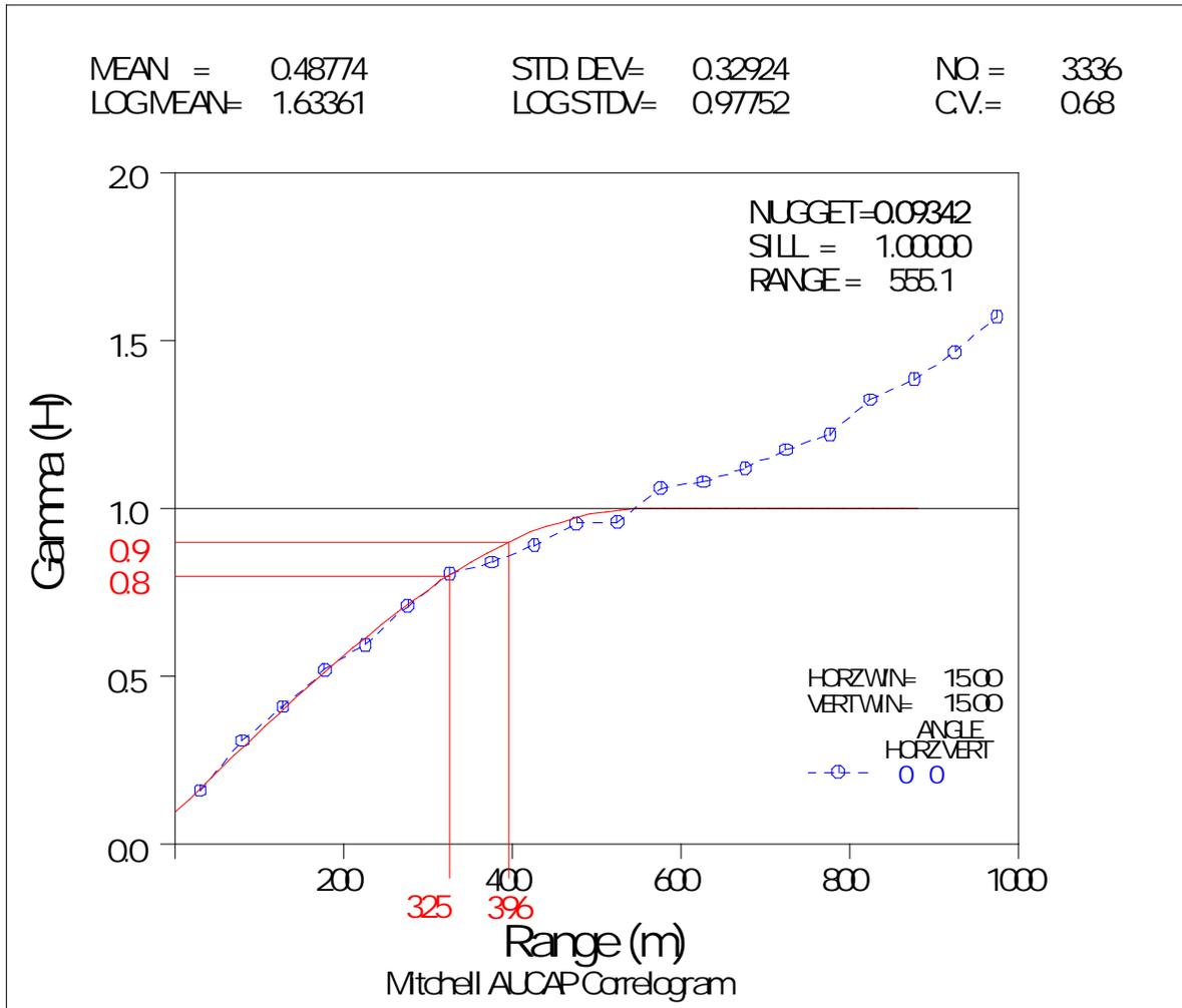
Figure 17-12: Iron Cap Au Grade Correlogram
