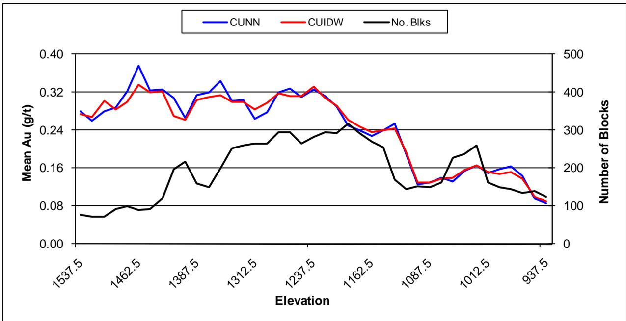
Figure 17-39: Mitchell Au-Cu Swath Plots by Elevation
