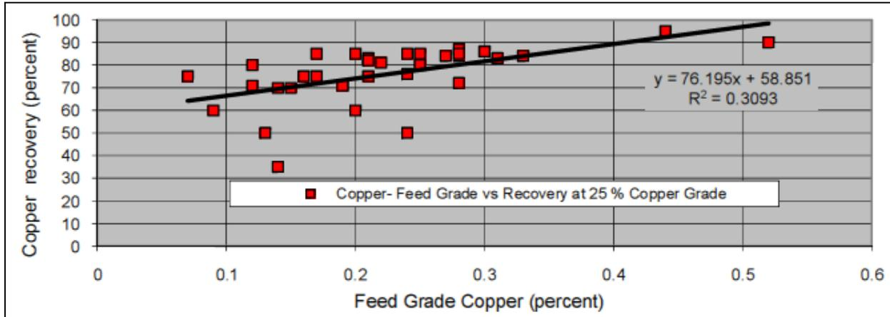
**Figure 16-3: Copper Recovery & Concentrate Grade – Individual Samples, Mitchell, 2008 (G&T)**
