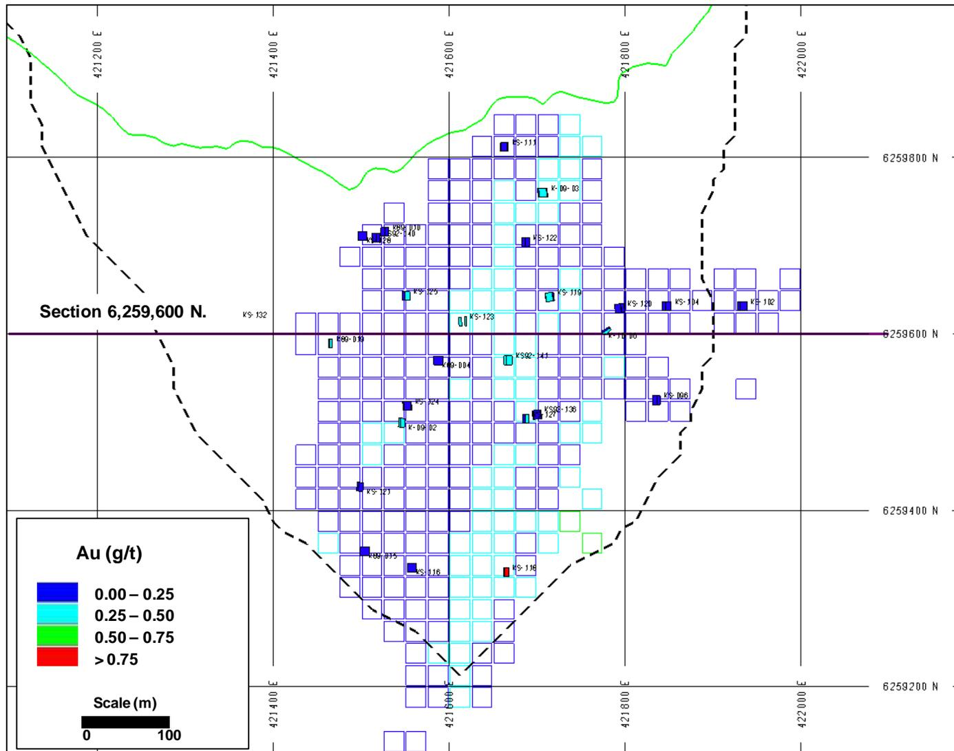
Figure 17-25: Sulphurets Au Block Model Cross Section 23
