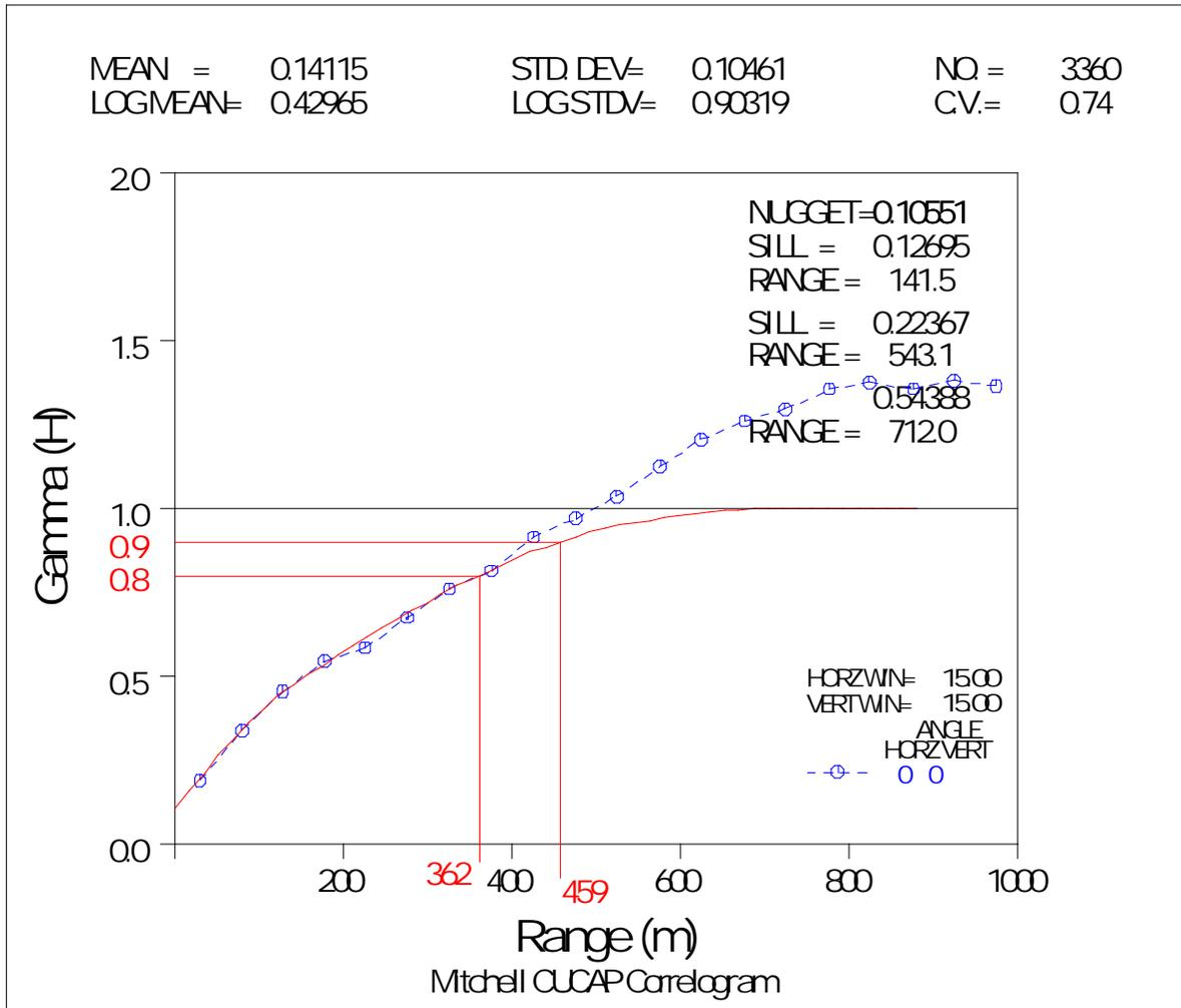
Figure 17-16: Iron Cap Cu Grade Correlogram
