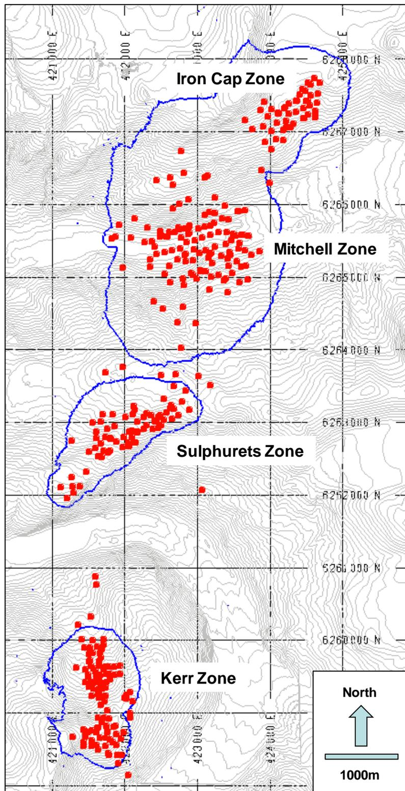
Figures 11-2 through 11-5 are drill hole collar maps for the Kerr, Sulphurets, Mitchell, and Iron Cap zones, respectively showing the collar location and hole trace in red. RMI's conceptual pits (pit number 3 as defined in Table 17-32) are shown in blue. For reference purposes, each drill hole collar map contains a reference line of section line for drill hole and block model cross sections shown in Section 17.8.
