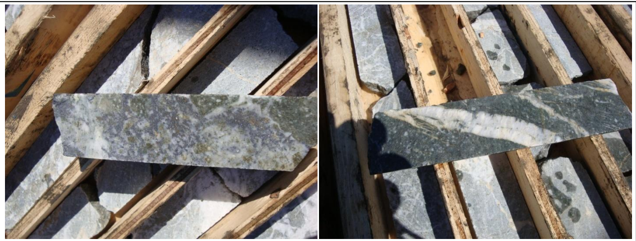
Figure 8-1. Silver Coin Project - Right, Low Sulphide Mineralisation with Quartz Veining. Left High Sulphide Mineralisation with Silification.
