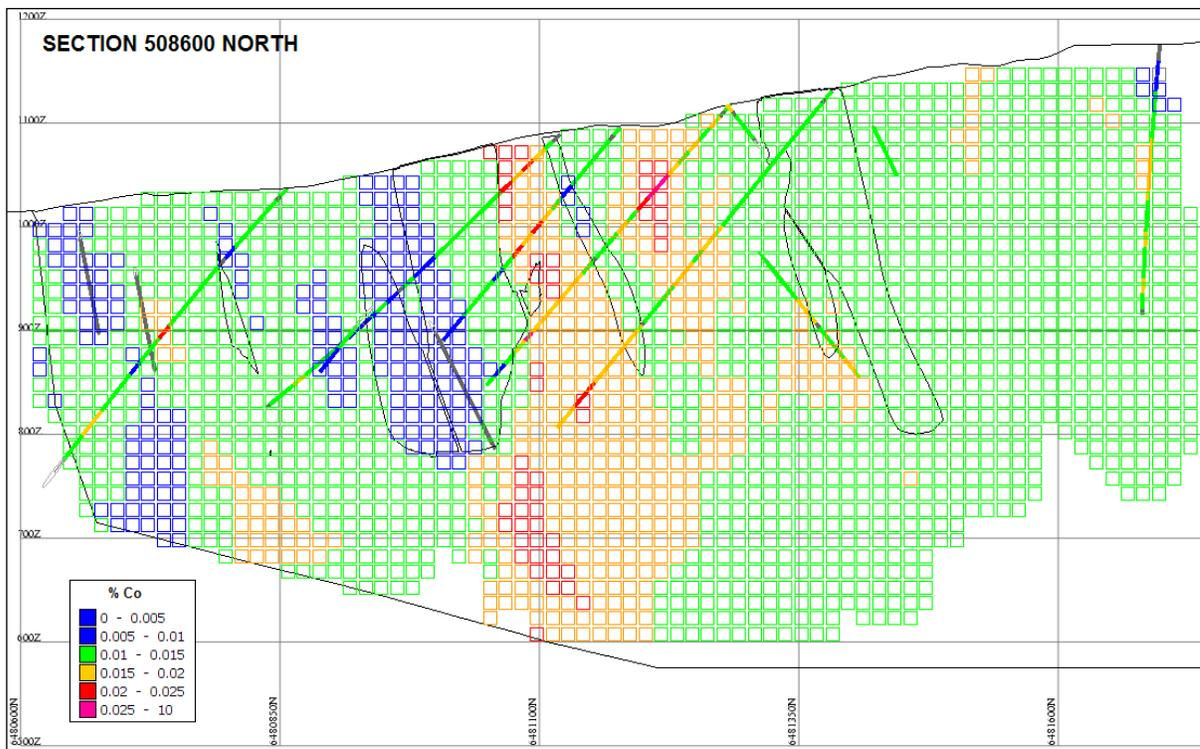
Figure 14.5 Section 508600 E - S Grades in Composites and Block Model
