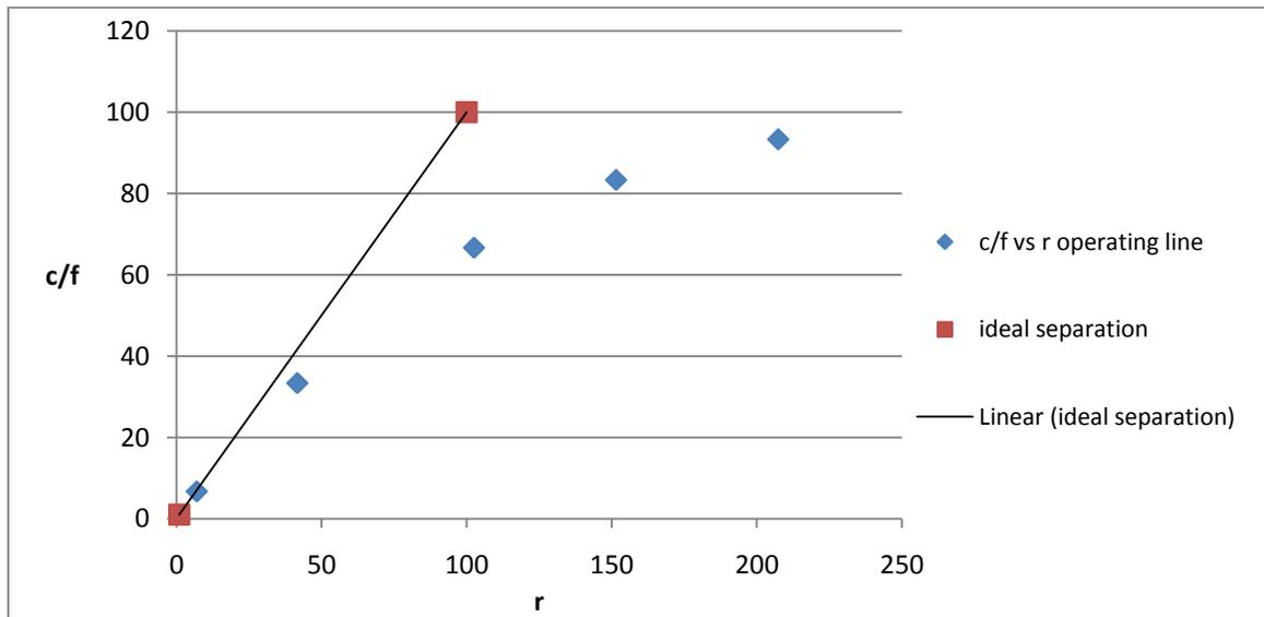
This equation is not solvable analytically, but from a body of data at various feed grades such as the grade-recovery data already derived, the model constant  $k$  can be determined iteratively by a minimization of the sum of the squares approach. The lower the value of  $k$  the better the separation i.e. on a superior grade-recovery curve. Once  $k$  is determined then the concentrate grades and recoveries at various feed grades can be calculated using goal seek in Excel.
