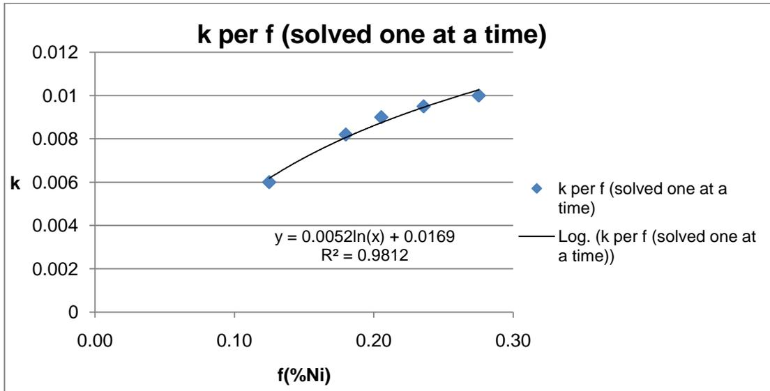
Applying this to an array of data with varying feed grades and a range of concentrate grades and solving the separation equation for recovery using the Excel function Goal Seek yields the graph shown below in Figure 13.8
