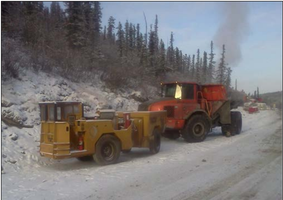
Figure 16.26: Young's 470 TZ Haul Truck (6.4-tonne capacity) (Volvo AE30 in background) (SRK, 2013)
