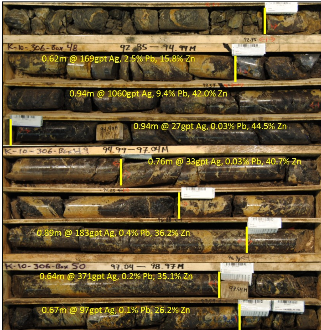
Figure 7.8: Vein-Fault Intercept in Drill Hole K-10-0306, in the Onek Deposit (Alexco, 2014)
