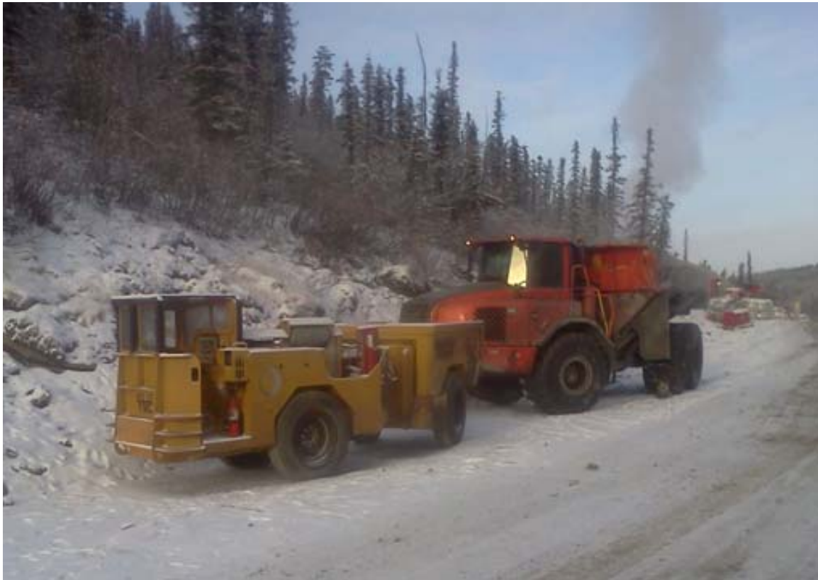
Figure 16-27: Young's 470 TZ Haul Truck (6.4-tonne capacity) (Volvo AE30 in background) (SRK, 2013)
