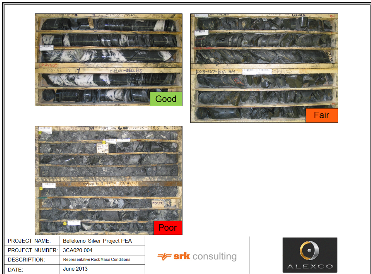
Figure 16-6: Representative Rock Mass Conditions Used for Core Re-Logging and Development of Geotechnical Domains (SRK, 2013)
