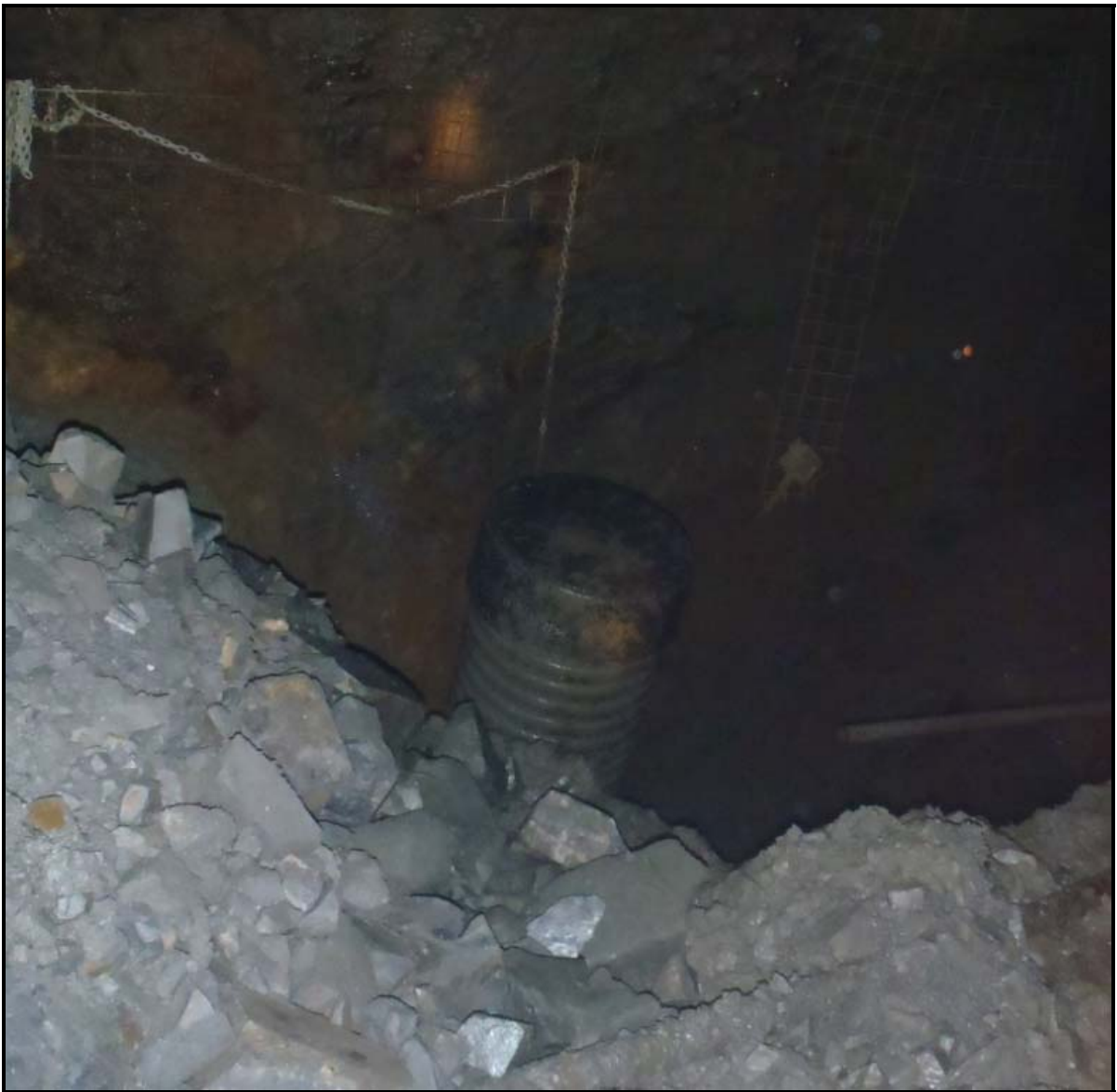
Figure 16-14: Culvert Installed in Longhole Stope (SRK, 2013)
