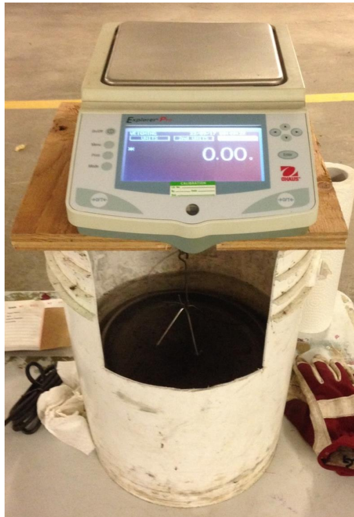
Figure 12-3 Balance scale and water bucket setup for measuring specific gravity of core
