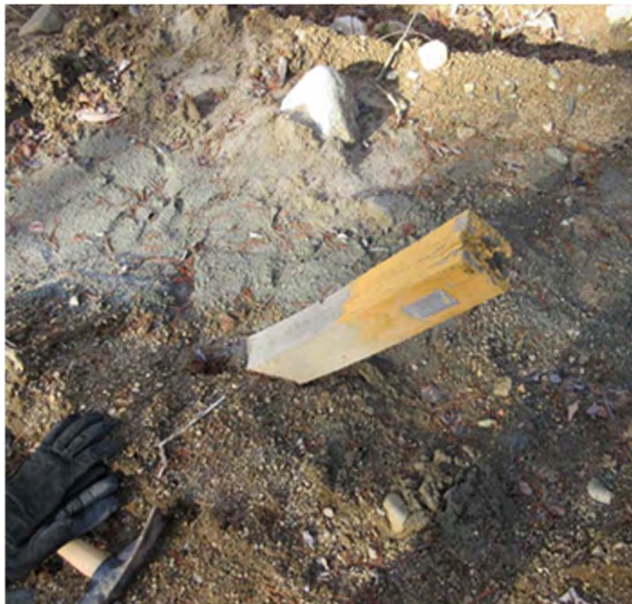
Figure 12.6: Collar marking for Drill Hole CN14-11
