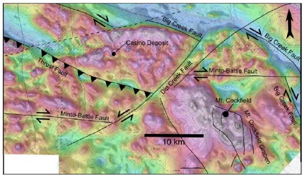
Figure 7-2: Regional structures overlain on recent aeromagnetic survey
