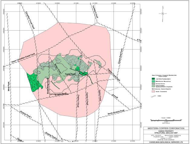
Figure 8-3: Casino Deposit Structural Geology Map
