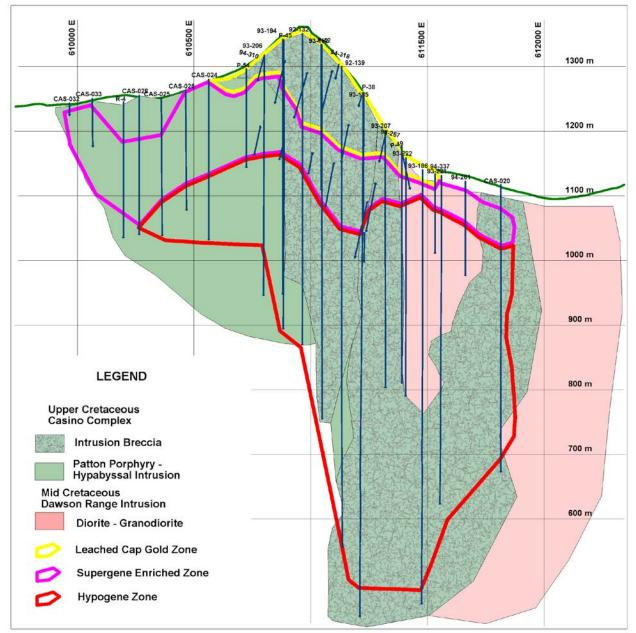
Figure 8-2: Casino Property Geology – Cross Section
